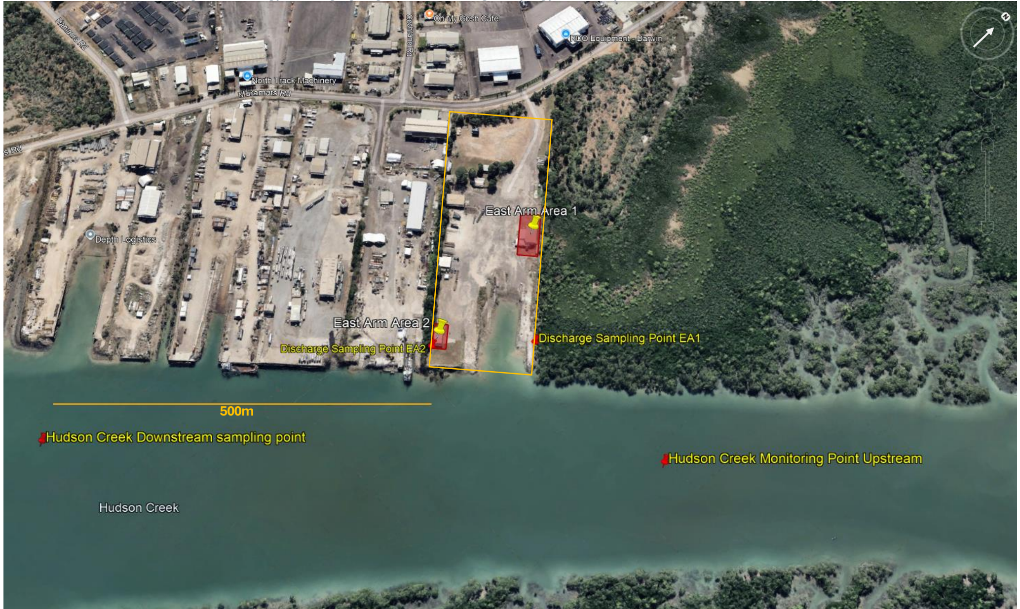
Image 4: Monitoring points– Highlighting two onsite discharge sampling points, the upstream and downstream monitoring points
