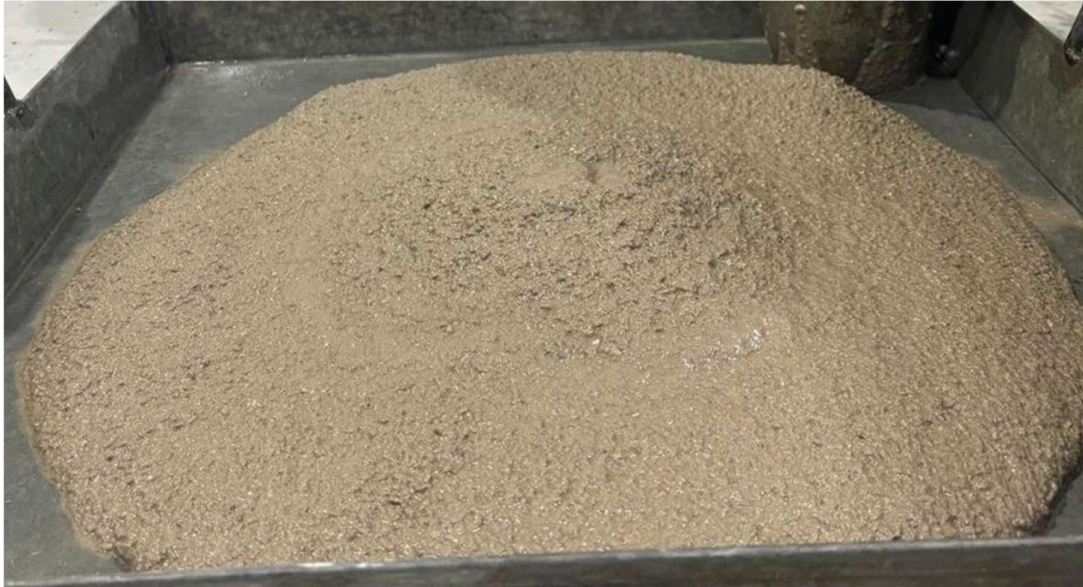
Figure 4.2: Paste Fill - Conical Slump at 80.0% Solids
