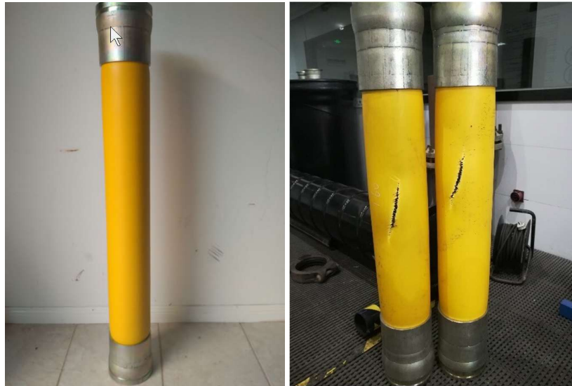
Figure 8.12: SRCP Burst Pipe
