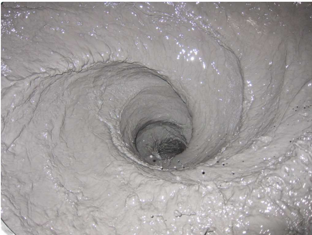
Figure 7.3: Vortex Mixer Slurry Action
