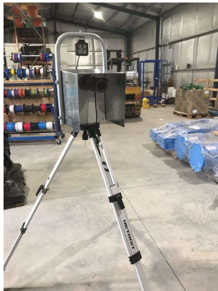
Figure 9.4: Camera Setup for Bulkhead Monitoring
