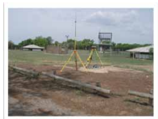
Figure 10 RTK GPS Reference Station
