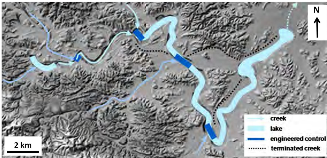
Figure 12. Closure landforms showing mine pit and flow-through pit lake (after Rio Tinto Iron Ore, 2011).
