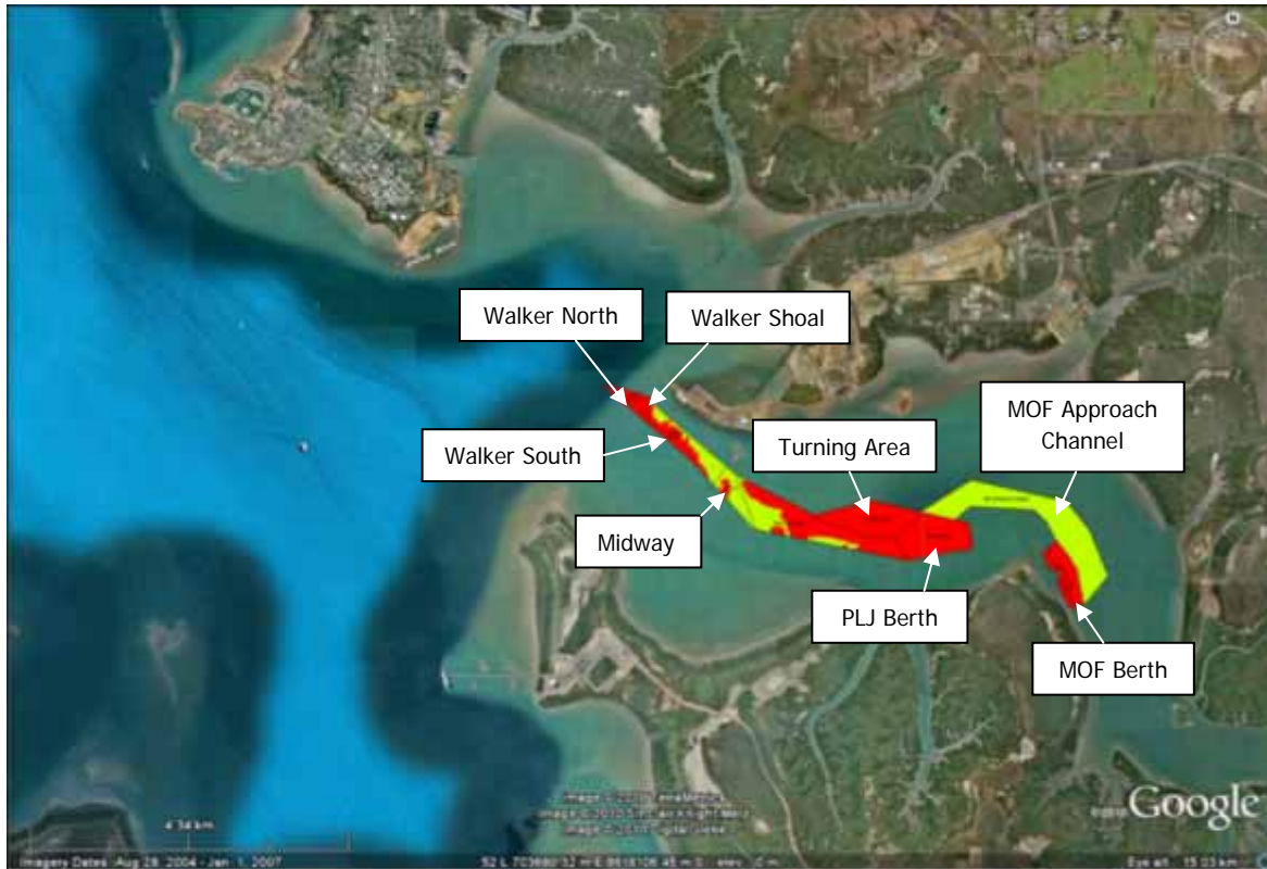
Figure 1-1 The proposed construction area in Darwin Harbour for the LNG infrastructure development. Red: area to be dredged; Green: area at/below required level.
