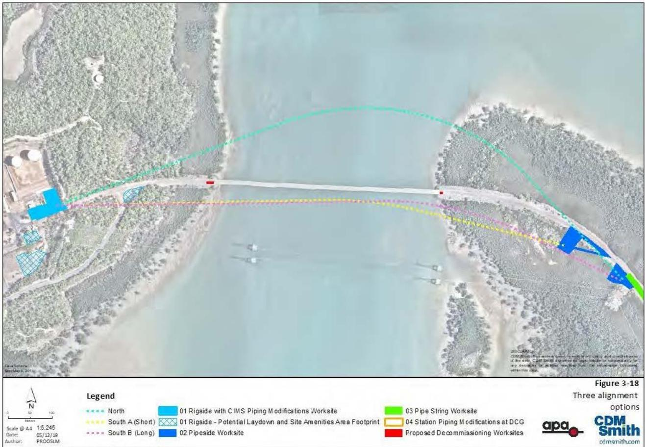
**Figure 1: Horizontal directional drill options (Source: Notice of Intent)**
