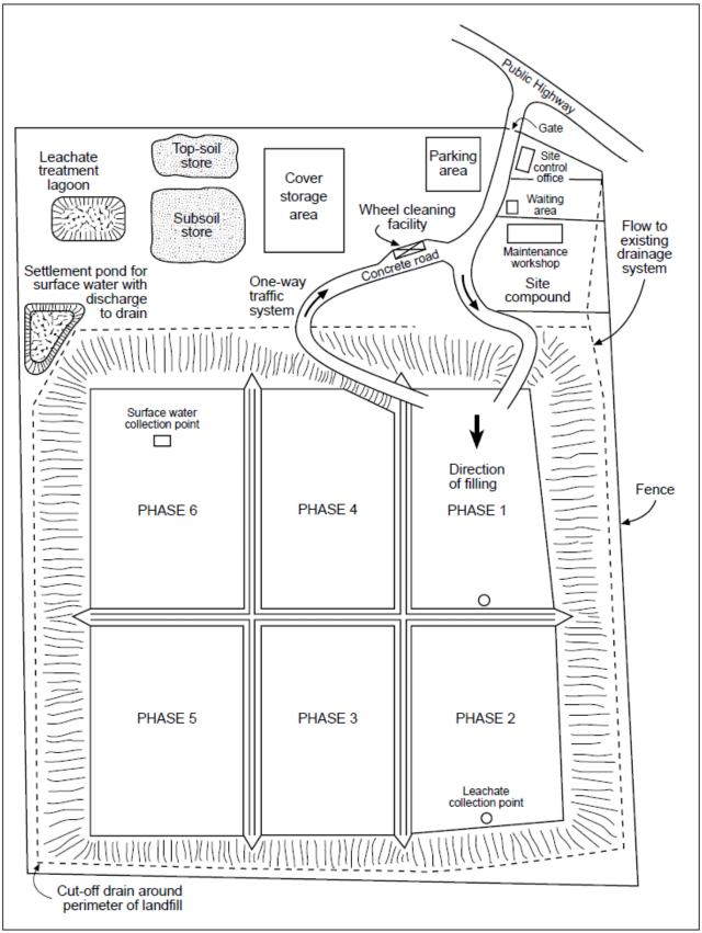
Figure 0.4: Typical Operational Plan for a Landfill Site<sup>5</sup>
