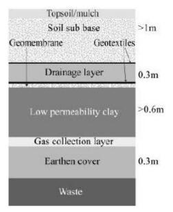
Figure 0.2: Indicative Landfill Cap Design<sup>7</sup>
