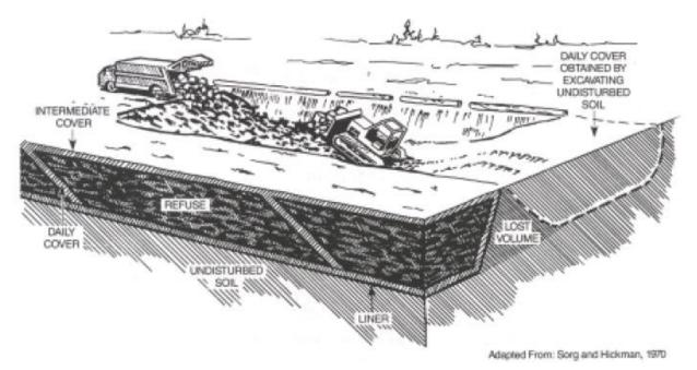
Figure 0.2: Trench Method of Landfilling<sup>3</sup>
