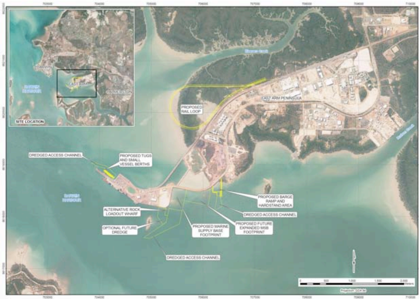
Figure 2 General Arrangement of the Proposed EAW Expansion (From Figure 5-1 Supplement – Proposed Rail Loop has now been removed from this Assessment)
