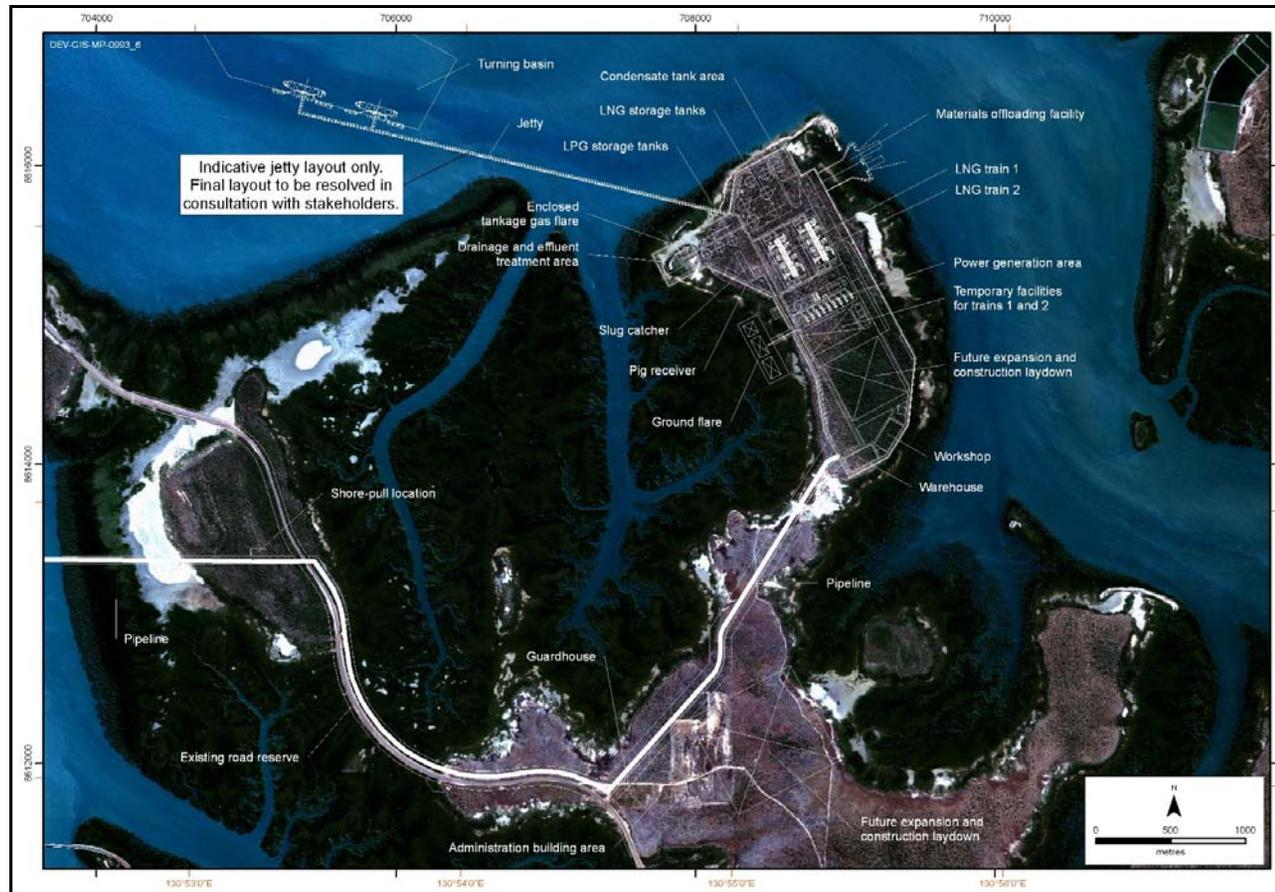
**Figure 3-5: Conceptual site plan for onshore gas-processing facility, onshore pipeline and MOF, at Blaydin Point**
