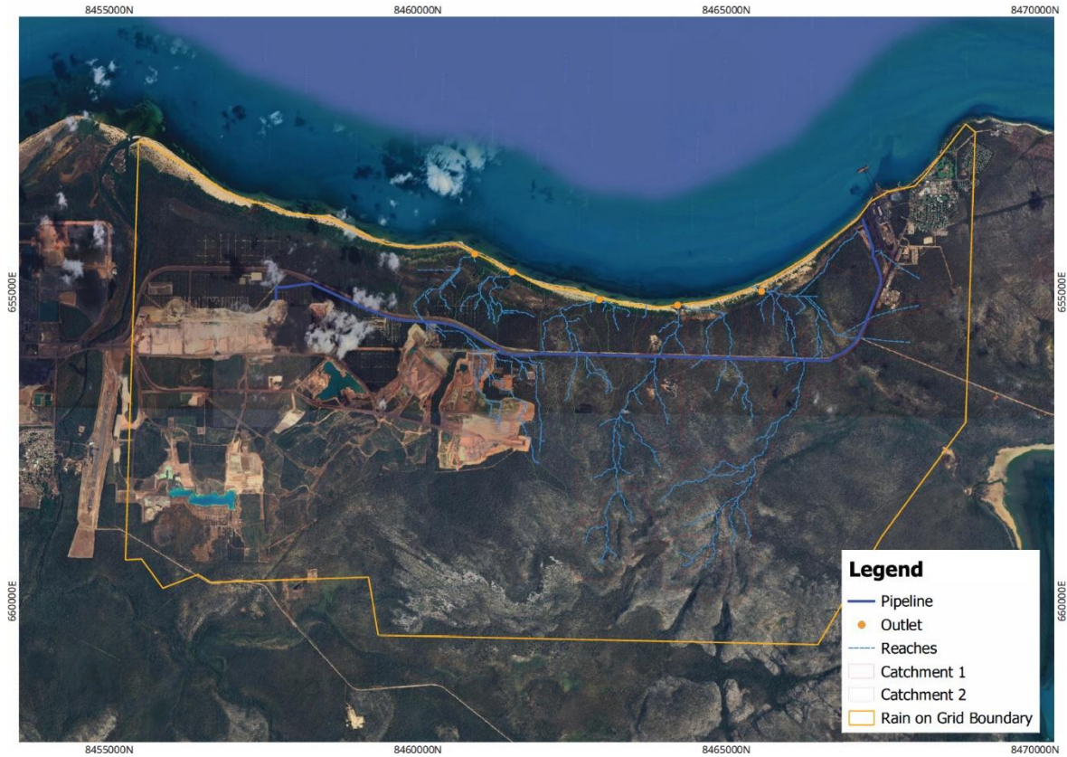
Figure 2: Catchment Delineation incorporating EWD Pipeline
