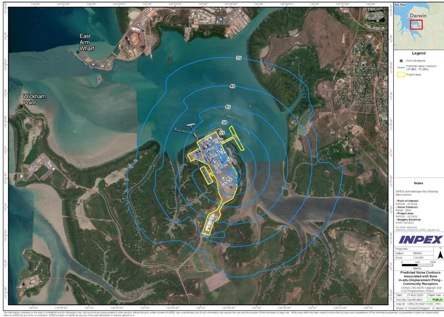
Figure 8-3: Worst-case noise propagation modelling for community receptors (Wood 2024)
