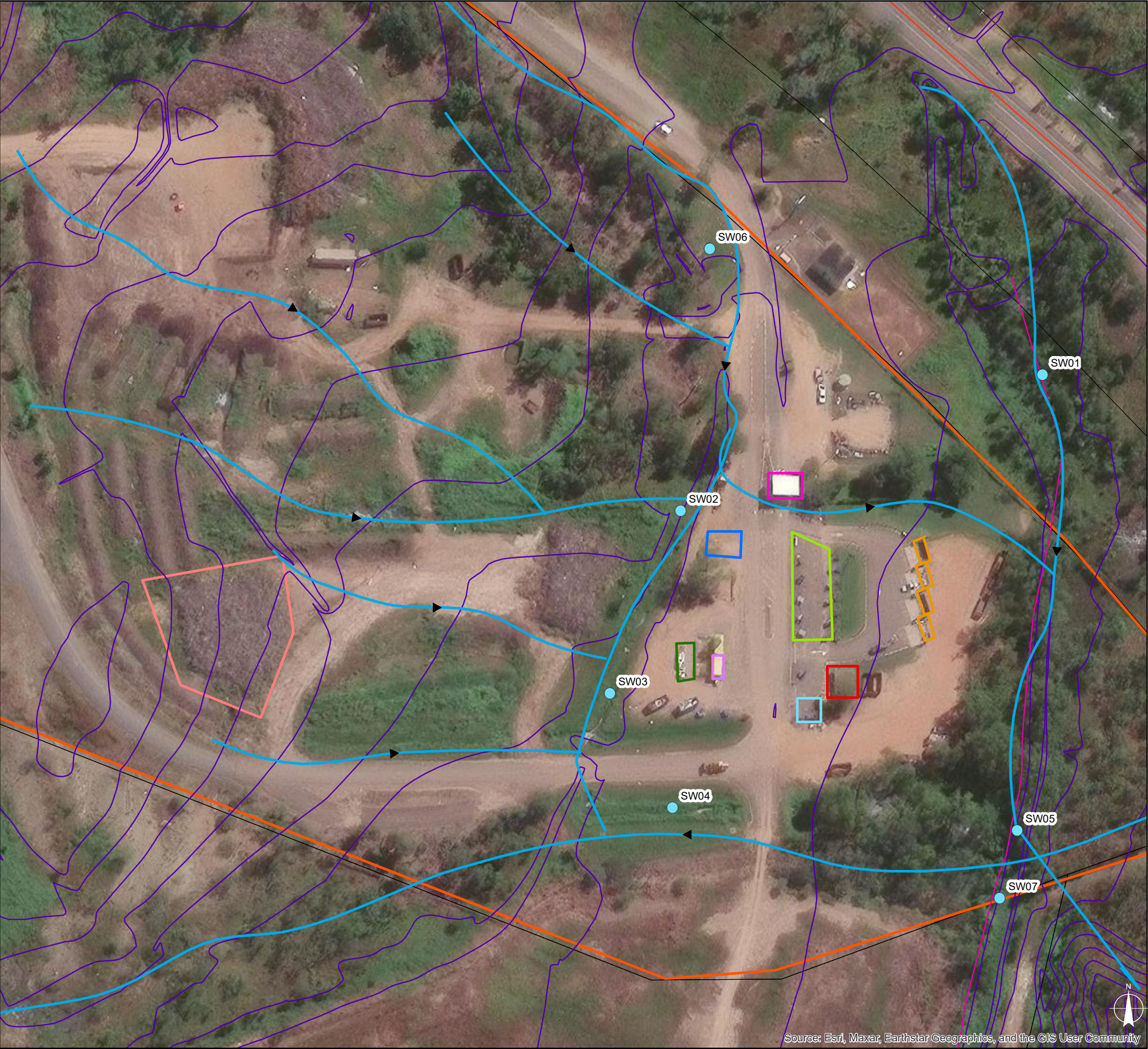
Archer Waste Facility Figure 1-2 Water pathways
