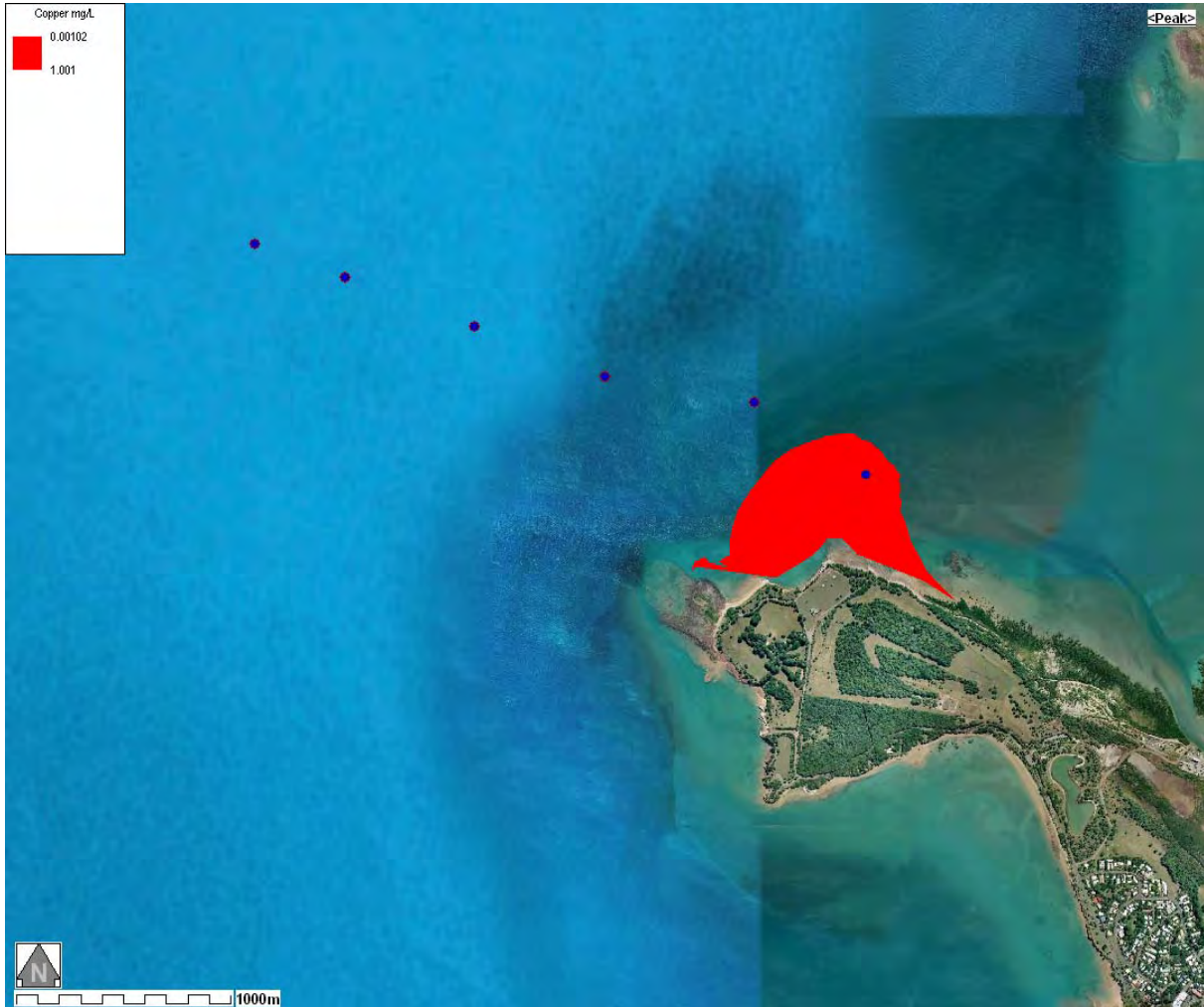
Plate 3-1 Typical dispersion model output for discharge from the existing EPO
