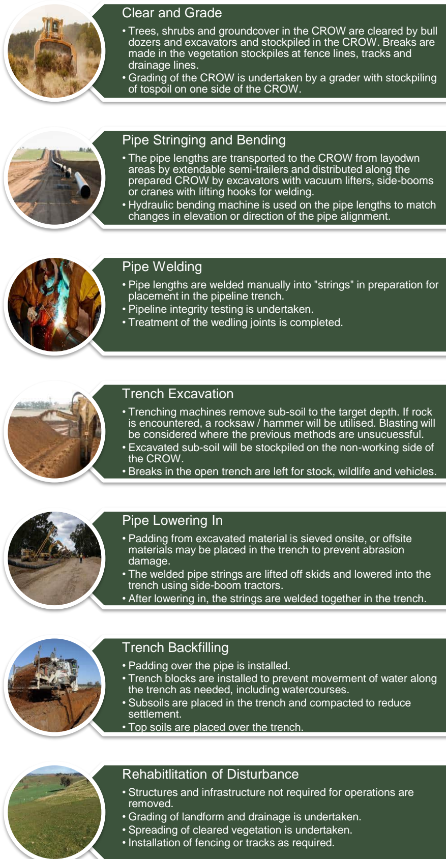
Figure 9: Stages of Trenched Pipeline Construction
