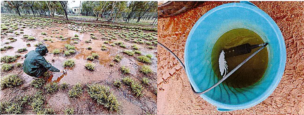
Figure 3 - Collecting surface water using a stainless steel cup (L) Bucket with collected water and YSI reader *
