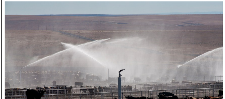
Plate 1 example of dust suppression sprays over stock pens
