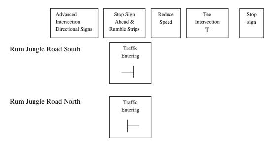
In addition guide posts should be installed at closer spacings on the Litchfield Park Road approach and the opposite side of Rum Jungle Road adjacent to the existing Direction Sign and Hazard Board. Rumble strips should also be considered for installation just prior to the Reduce Speed sign.
