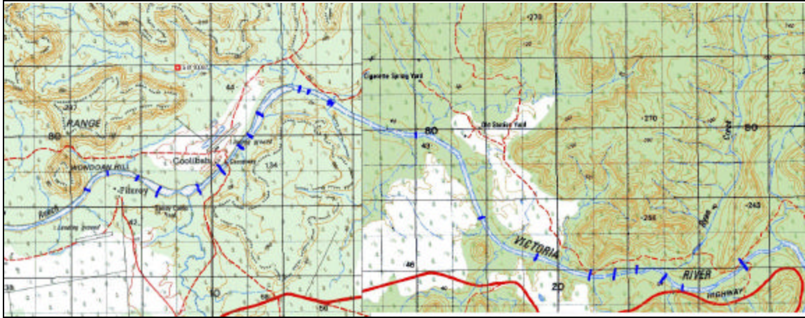
Figure 1 ADCP transects along the Victoria River from Coolibah upstream to the Victoria River roadhouse.
