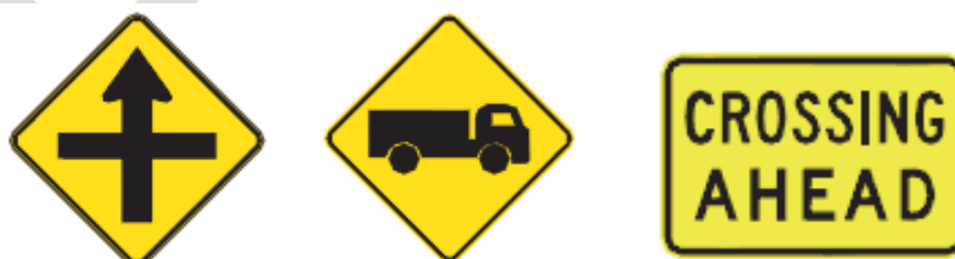
Figure 5.3 “Cross Road” (W2-1C), “Trucks” (W2-22C) and “Crossing Ahead” (W8-22C) signs
