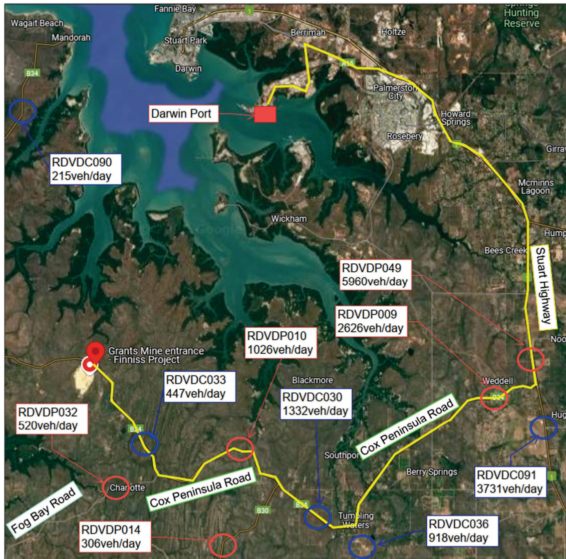
Figure 5 Count stations with the latest count volumes along Cox Peninsula Road (from NTG 2023 Annual Traffic Count Report)
