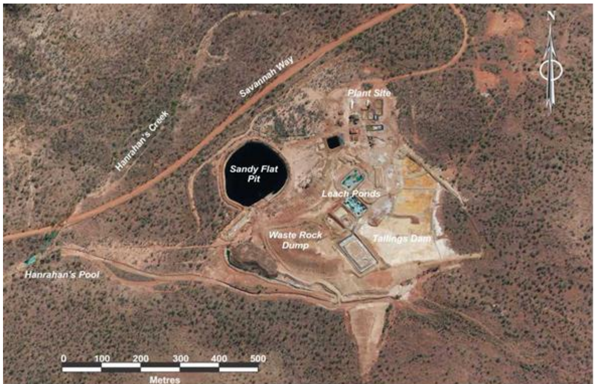
Figure 3: Redbank Mine Site showing Sandy Flat Pit, Waste Rock Dump, Leach Ponds and Tailings Storage Facility
