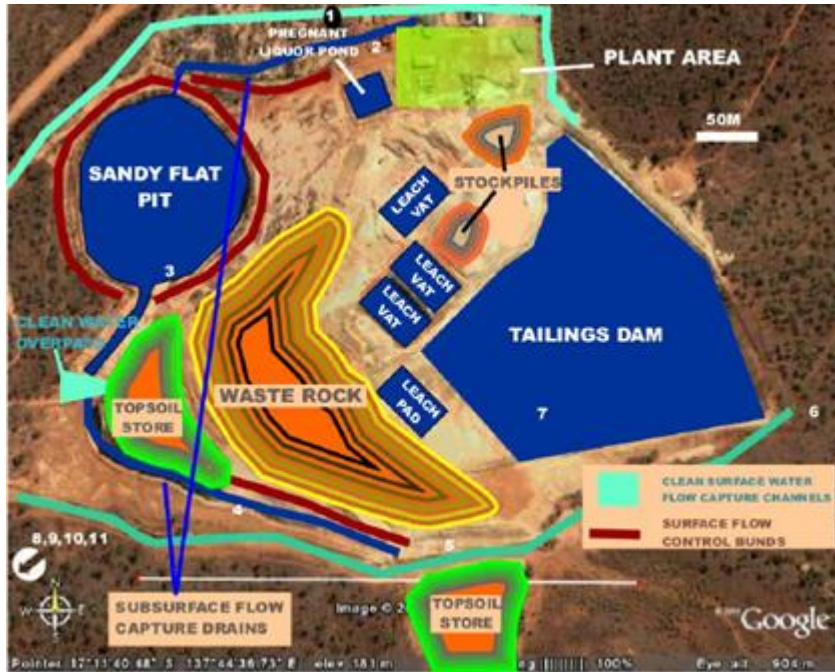
Figure 19: Redbank Mine Diversion Drainage works
