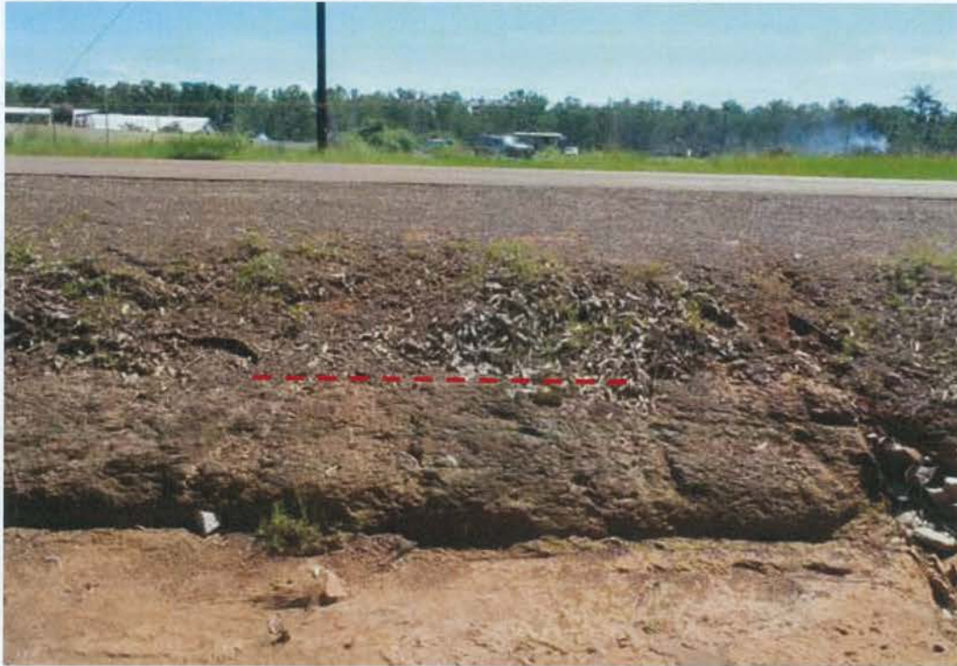
Photo 1: View of OUD on south side of Boulter Road showing laterite profile
