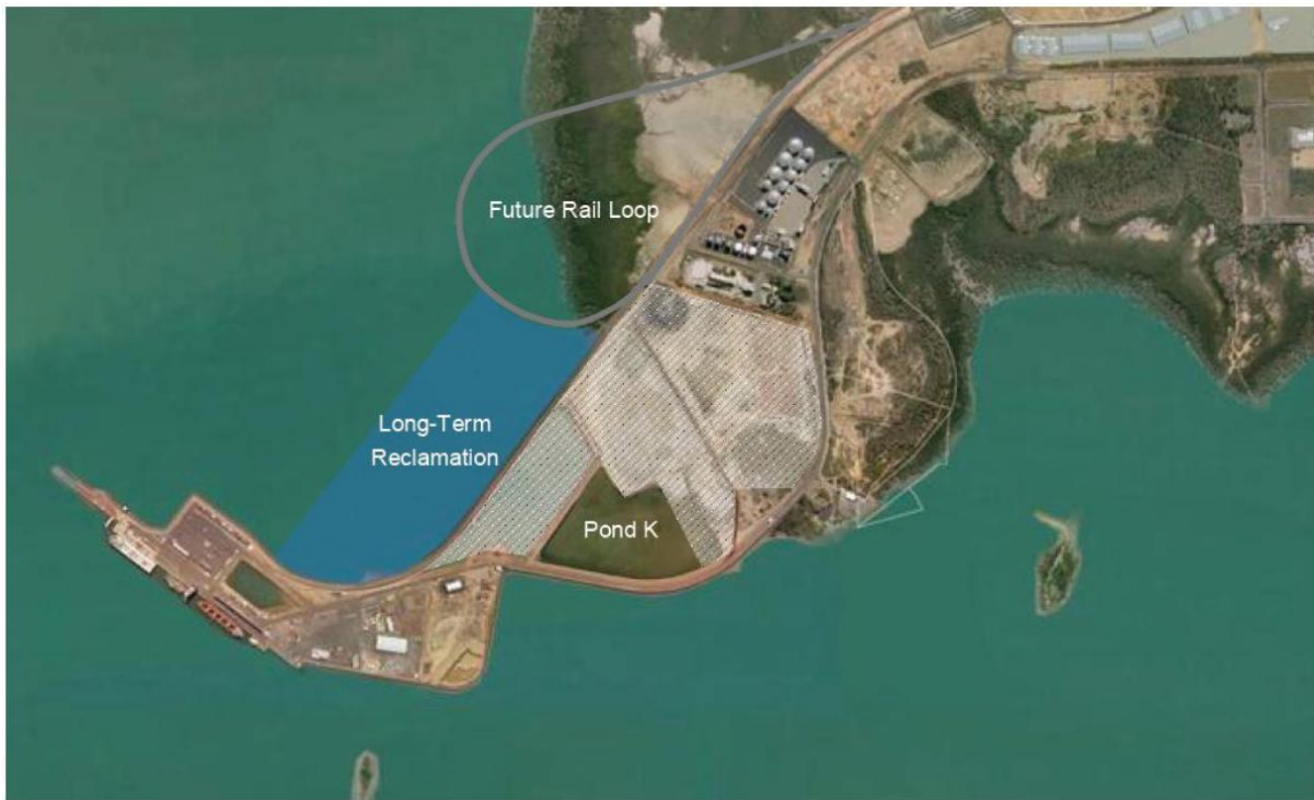
Figure A-3 Indicative Extent of Future Long-term Reclamation for Dredged Material (AECOM,2011)
