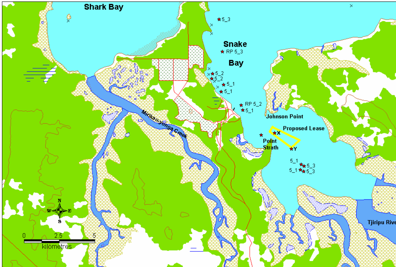
Figure 3-2 Deep water (5m) drogue survey showing positions of drogues during one spring tide cycle. Drogues to seaward of the farm site were released during the ebb tide at position X or the relevant RP site; those inland were released during the flood tide from point Y.
