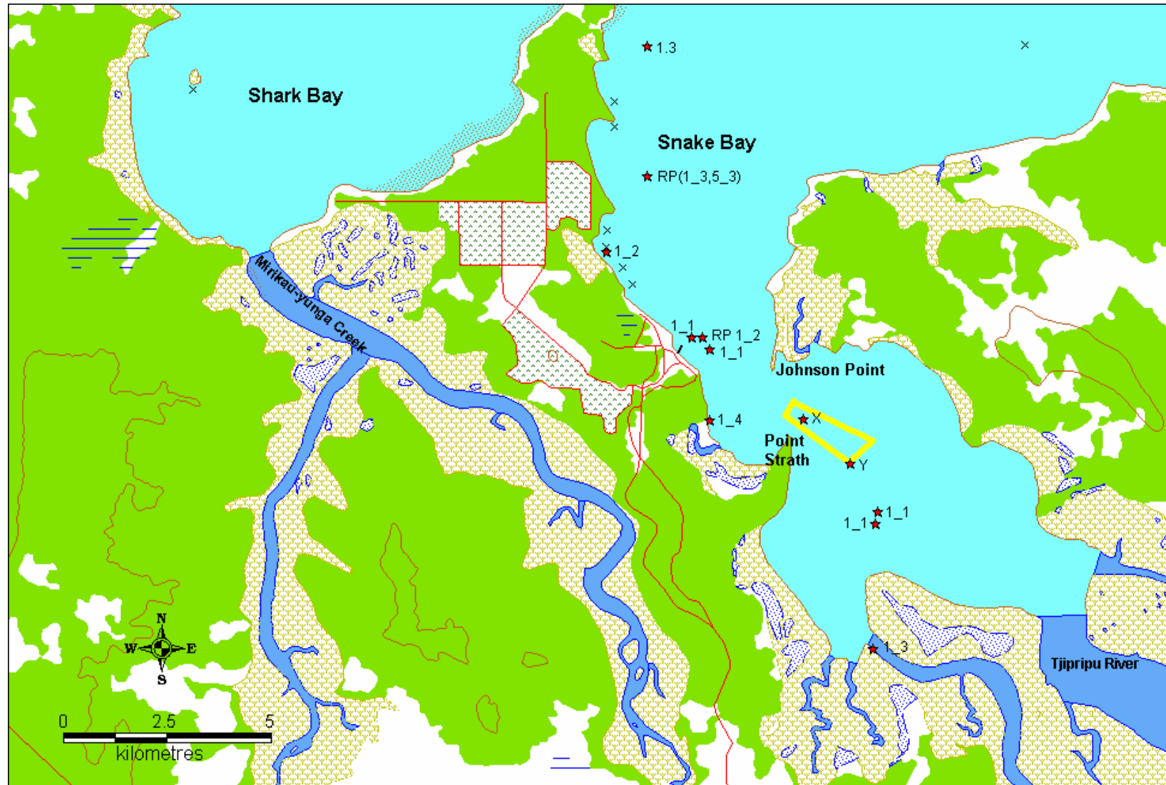
Figure 3-1 Shallow water (1m) drogue survey showing positions of drogues during one spring tide cycle. Drogues to seaward of the farm site were released during the ebb tide at position X or the relevant RP site; those inland were released during the flood tide from point Y.
