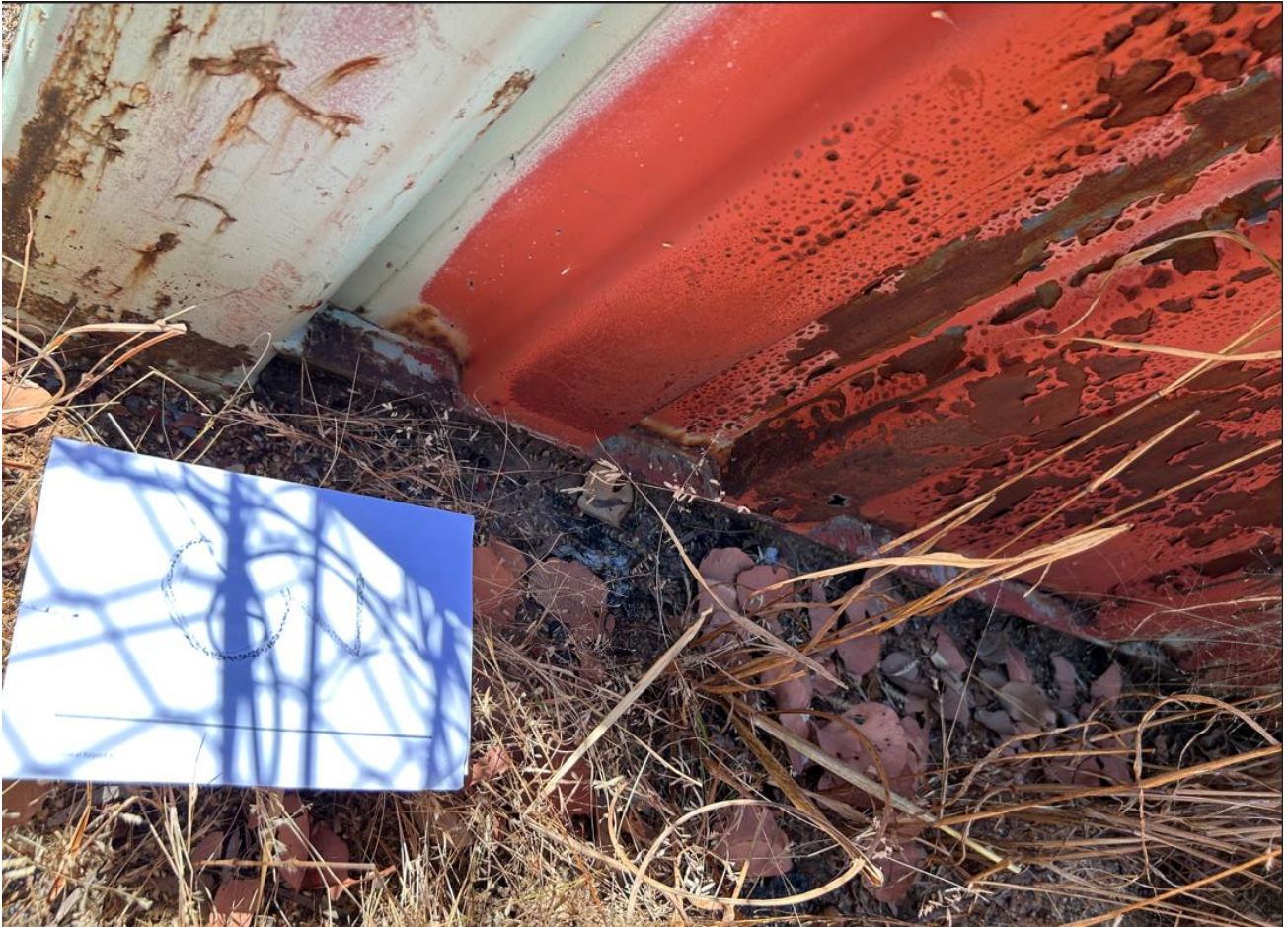
Figure 34. Close up of degradation along inside long side of container #3, where samples are potentially spilling out
