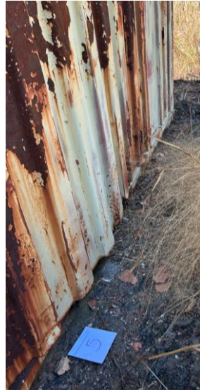
Figure 47a. Buckling of the side wall on container 5, integrity of the container has been breached along the bottom. b) and side c) Close up of rust along the wall looking towards the end of the container.
