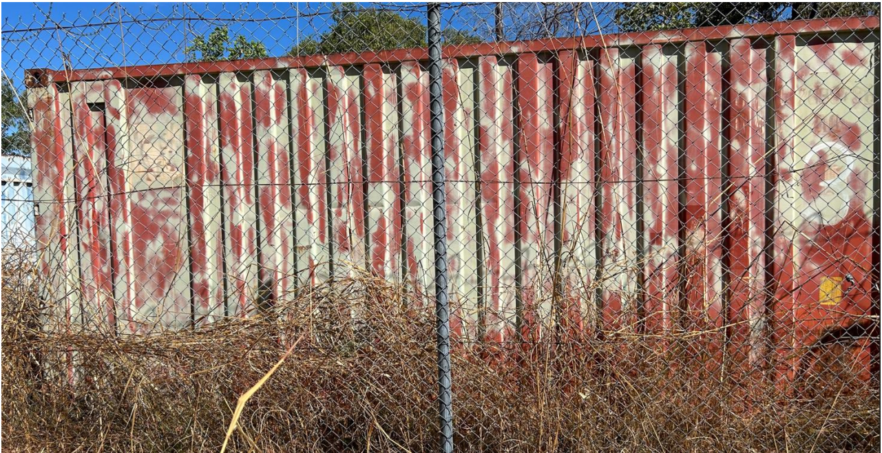
Figure 34. Close up of degradation along inside long side of container #3, where samples are potentially spilling out
