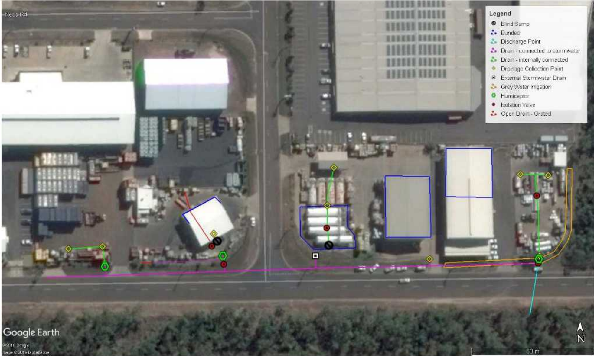
Figure 2 OEG Offshore facility surface water drainage network
