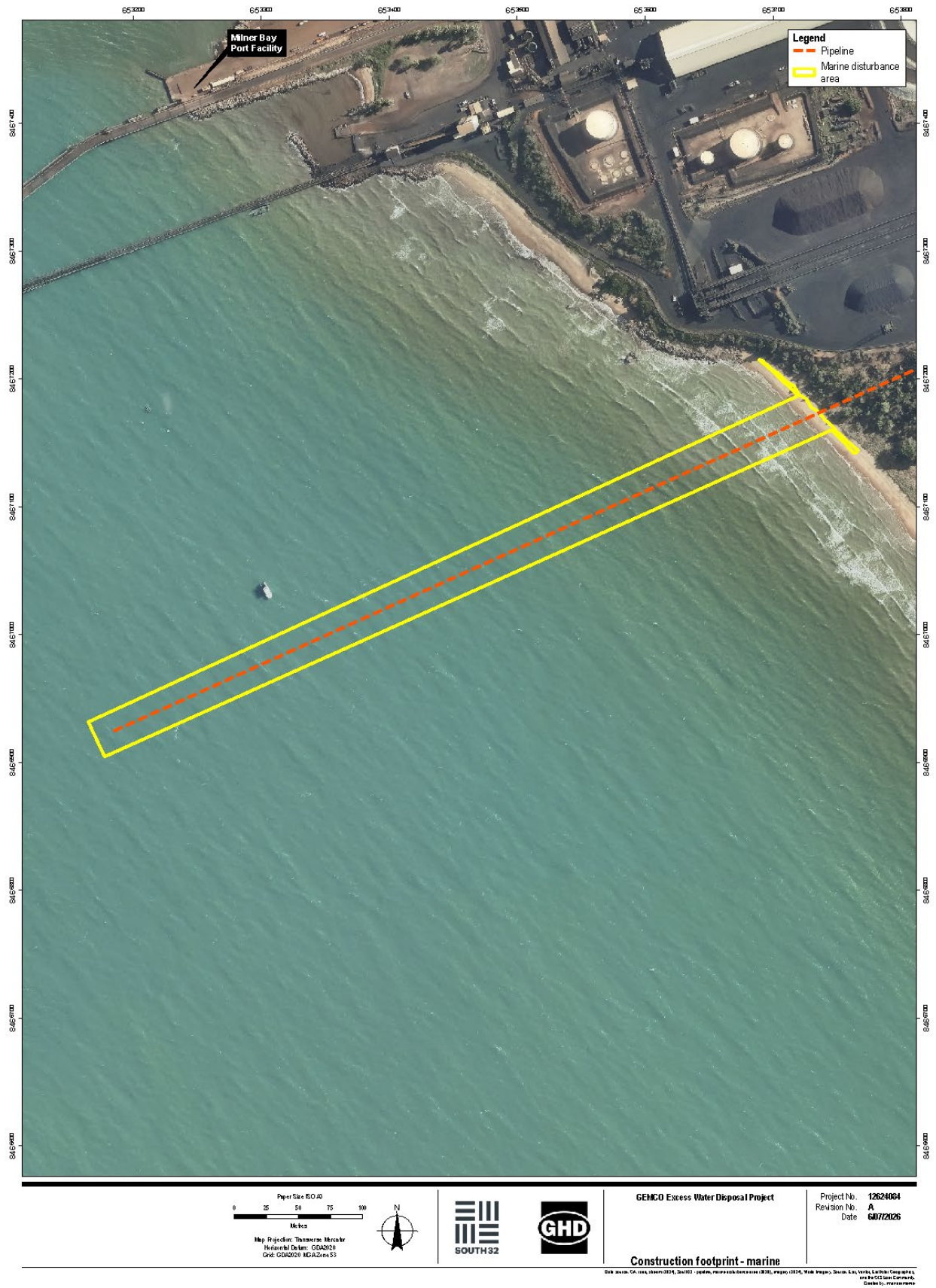
Figure 2 - Marine disturbance area approved extent and alignment
