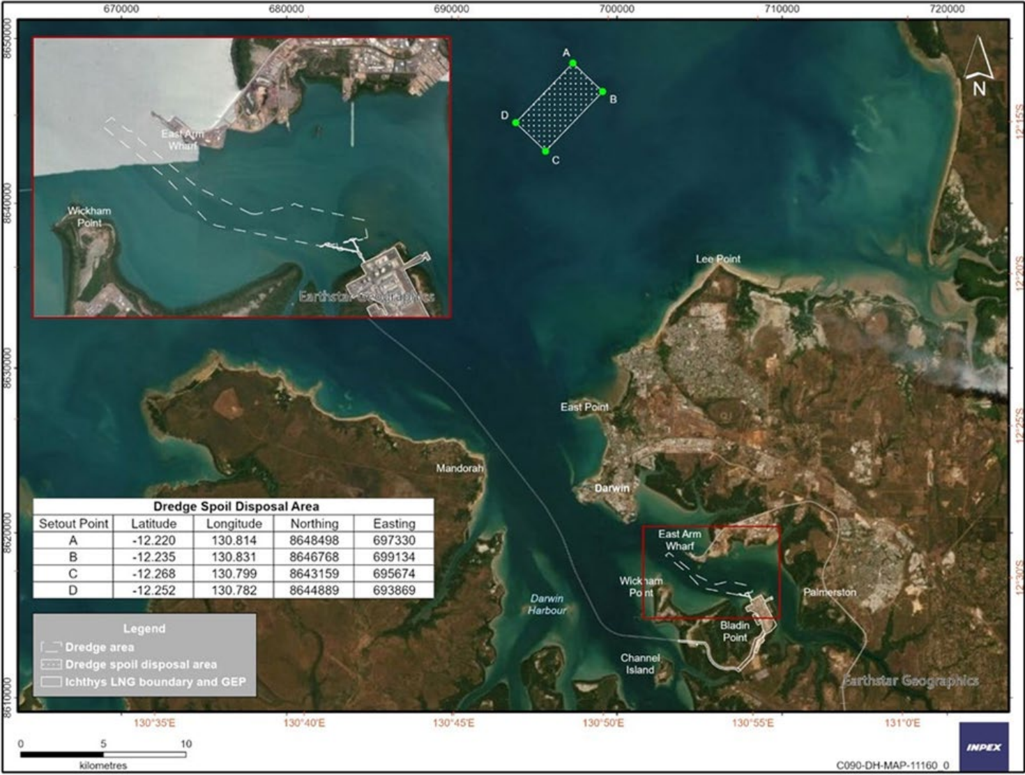
Figure 1. Location and approved extent of dredge footprint and dredge spoil disposal area (Source: Draft DMP, Appendix A of the referral)
