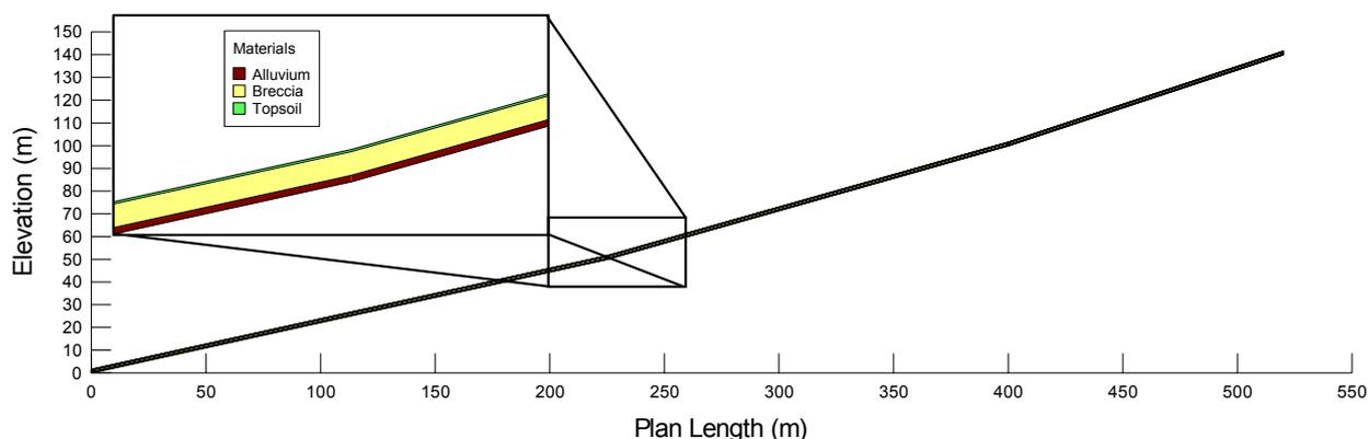
Figure 3-1: Geometry used to simulated 2D SPA model of Base-Case Batter Cover System.
