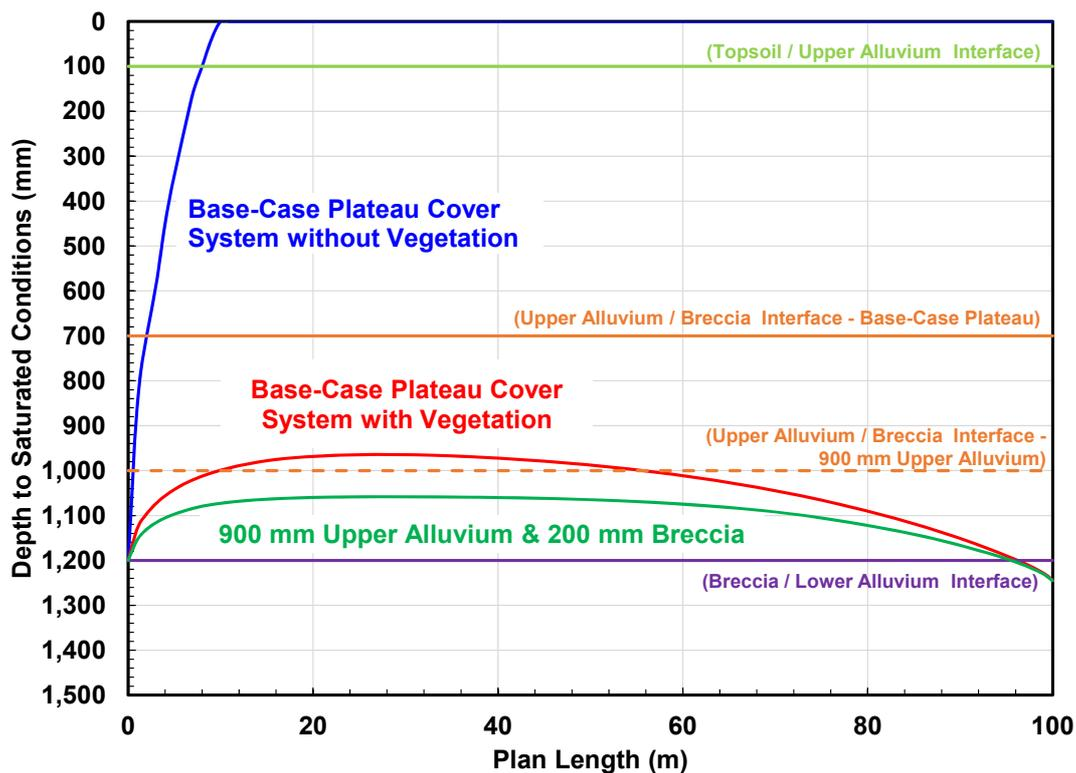
Figure 4-3 : Depth to saturation within the plateau cover system versus slope position.
