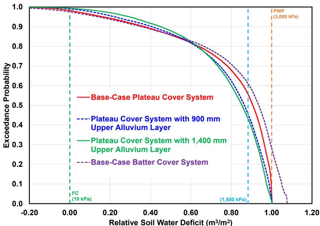
Figure 4-1 : Exceedance probability graph for soil water deficit predicted within cover systems.
