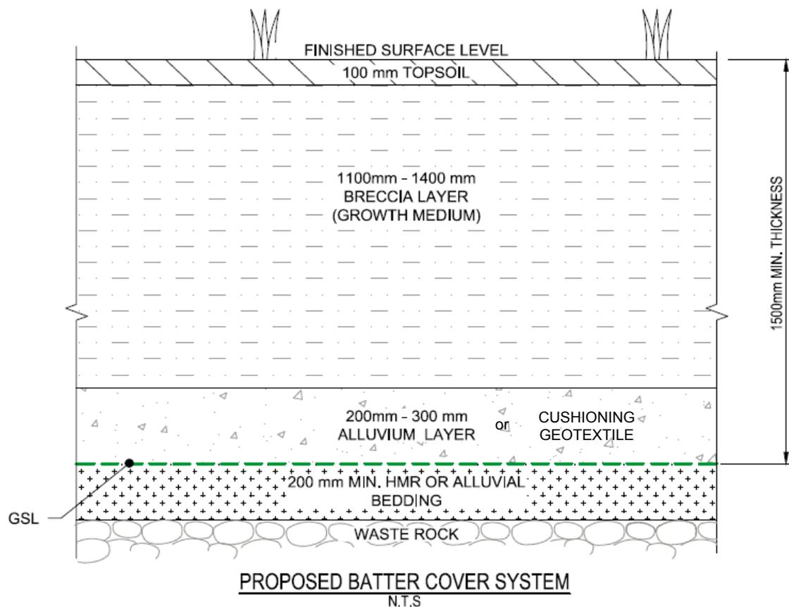
Figure 6-1: Proposed batter cover system profile
