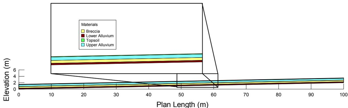
Figure 3-2: Geometry used to simulated 2D SPA model of Base-Case Plateau Cover System
