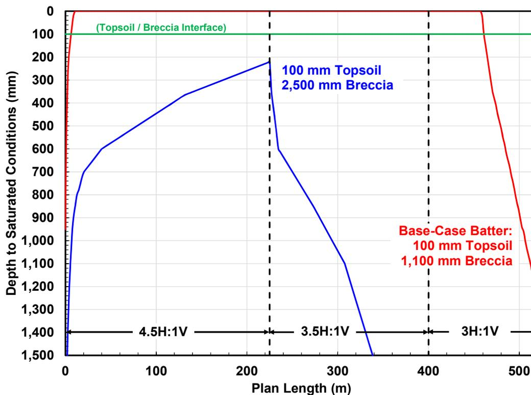
Figure 4-2: Depth to saturation within the batter cover system versus slope position.
