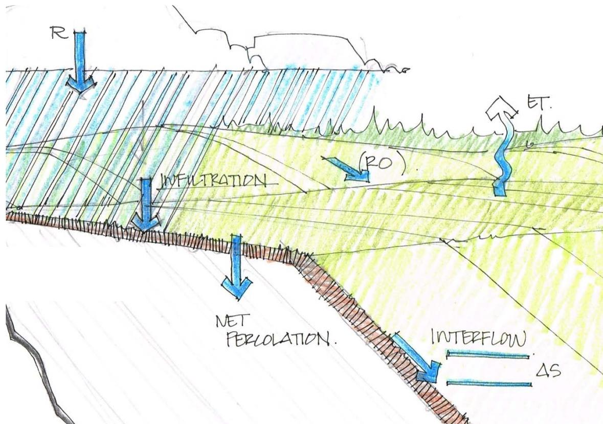
Figure 2-1: Schematic of hydrologic processes that influence performance of sloping cover systems for waste rock.
