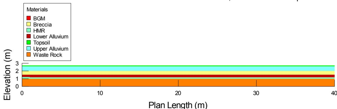
Figure 3-3: Geometry used to simulate a quasi-3D SPA model of the Base-Case Plateau Cover System.
