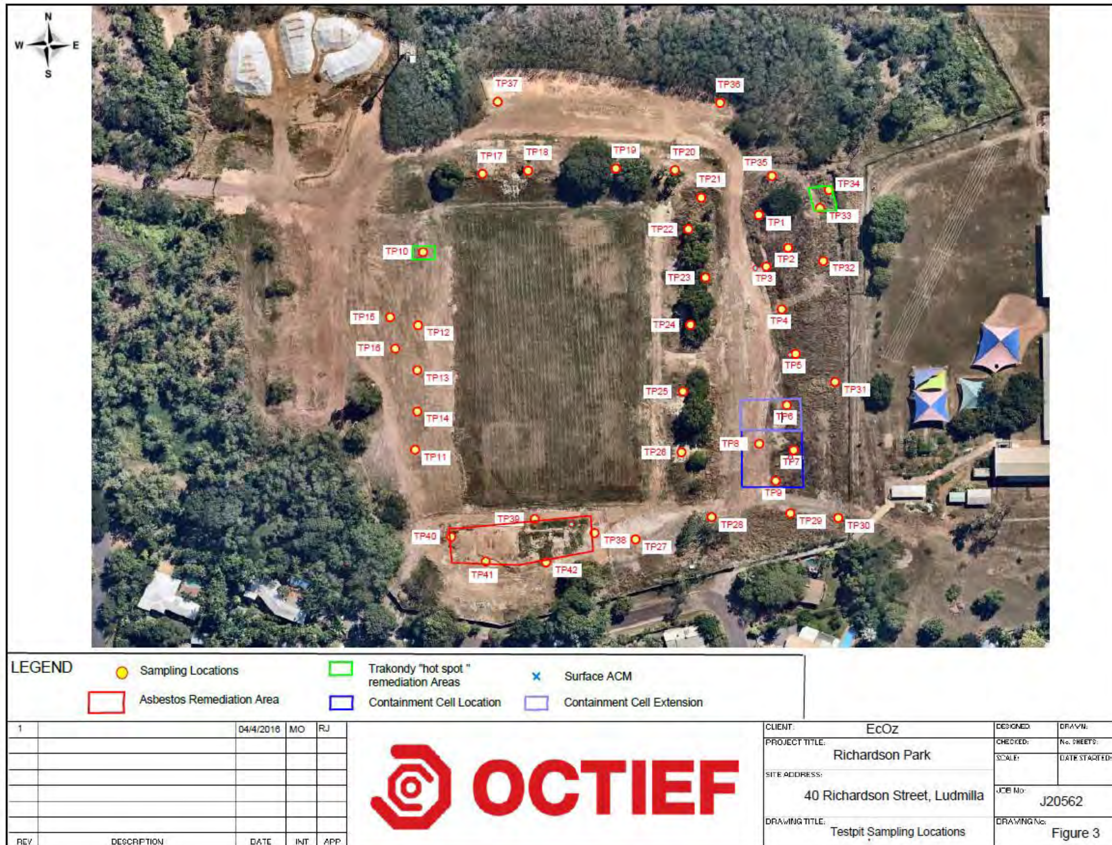
Figure 7: Supplementary investigation (test pit locations), Octief (2022)
