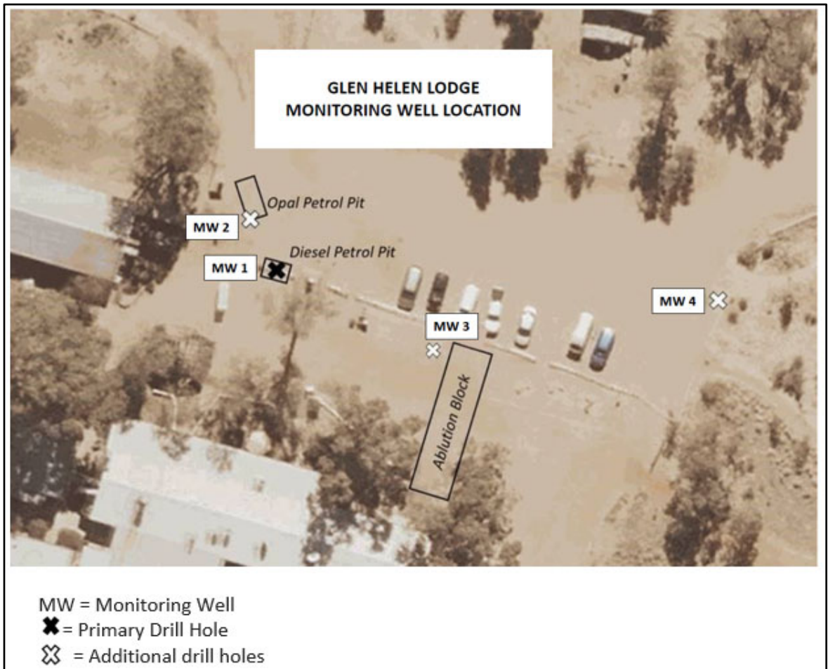
Figure 13. Test Locations – Groundwater bore locations (Low Ecological, 2022)
