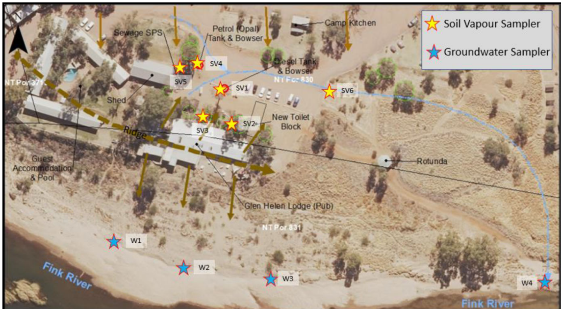
Figure 12. Test Locations – Soil vapour bores and surface water samples, September 2021 (Low Ecological, 2022)
