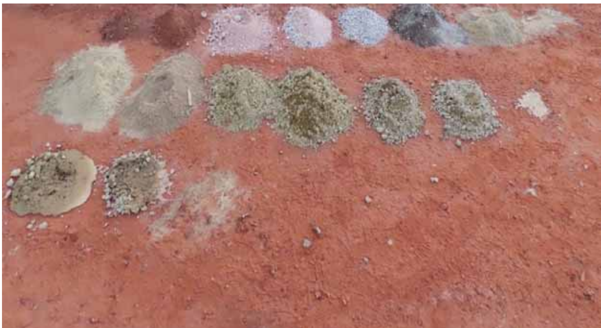
Figure 4: Samples of the rock-portfolio taken during the drilling of MW 2 (Opal petrol pit). From left to right, back to front: Top layer (backfill), grey rock quartz, white is silt stone, yellow clay, yellow clay moist, water quartz sandstone.
