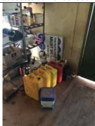
Photo: Chemical/flammables stored in maintenance shed on floor and shelf.
