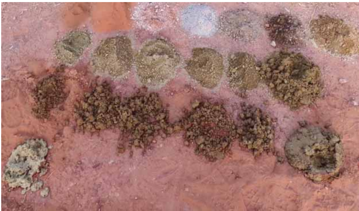
Figure 6: Samples of the rock-portfolio taken during drilling of MW 4. From left to right, back to front: Top layer (backfill), grey rock quartz, loose yellow clay, yellow clay, water rock.
