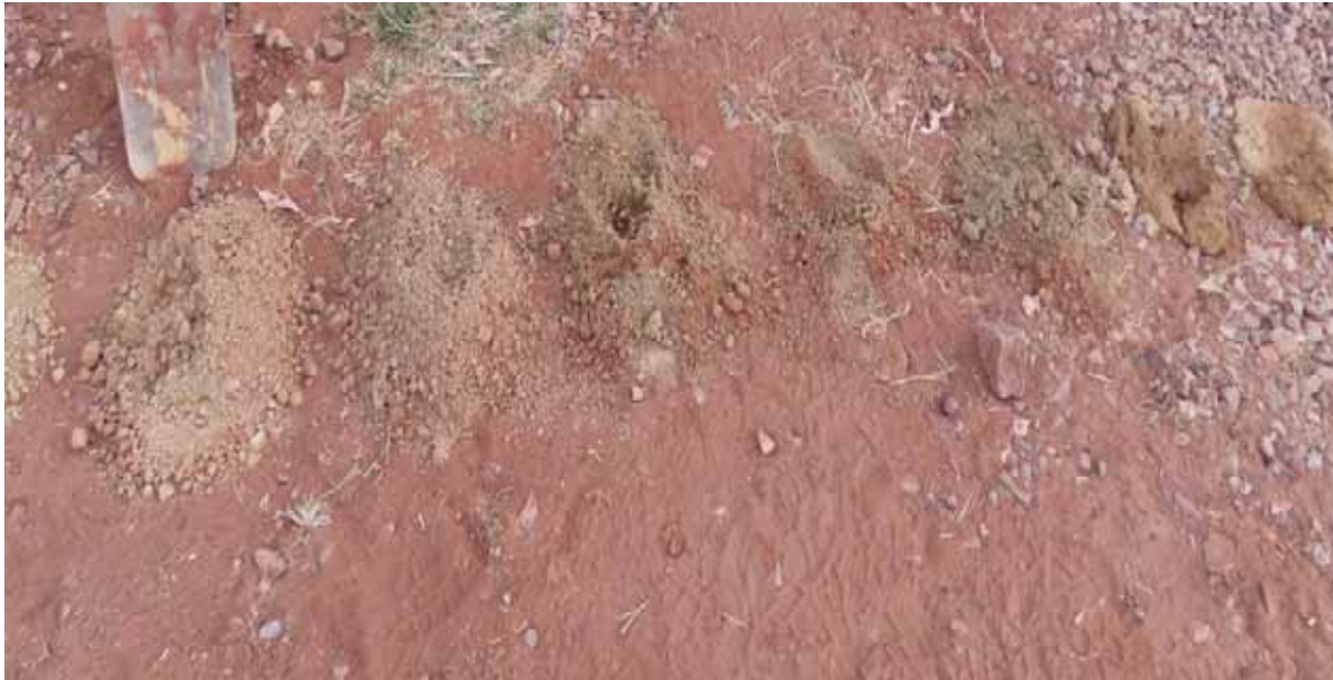
Figure 3: Samples of the rock-portfolio taken during drilling MW1. These soil samples belong to the old diesel petrol pit and show mostly rock and yellow claystone.
