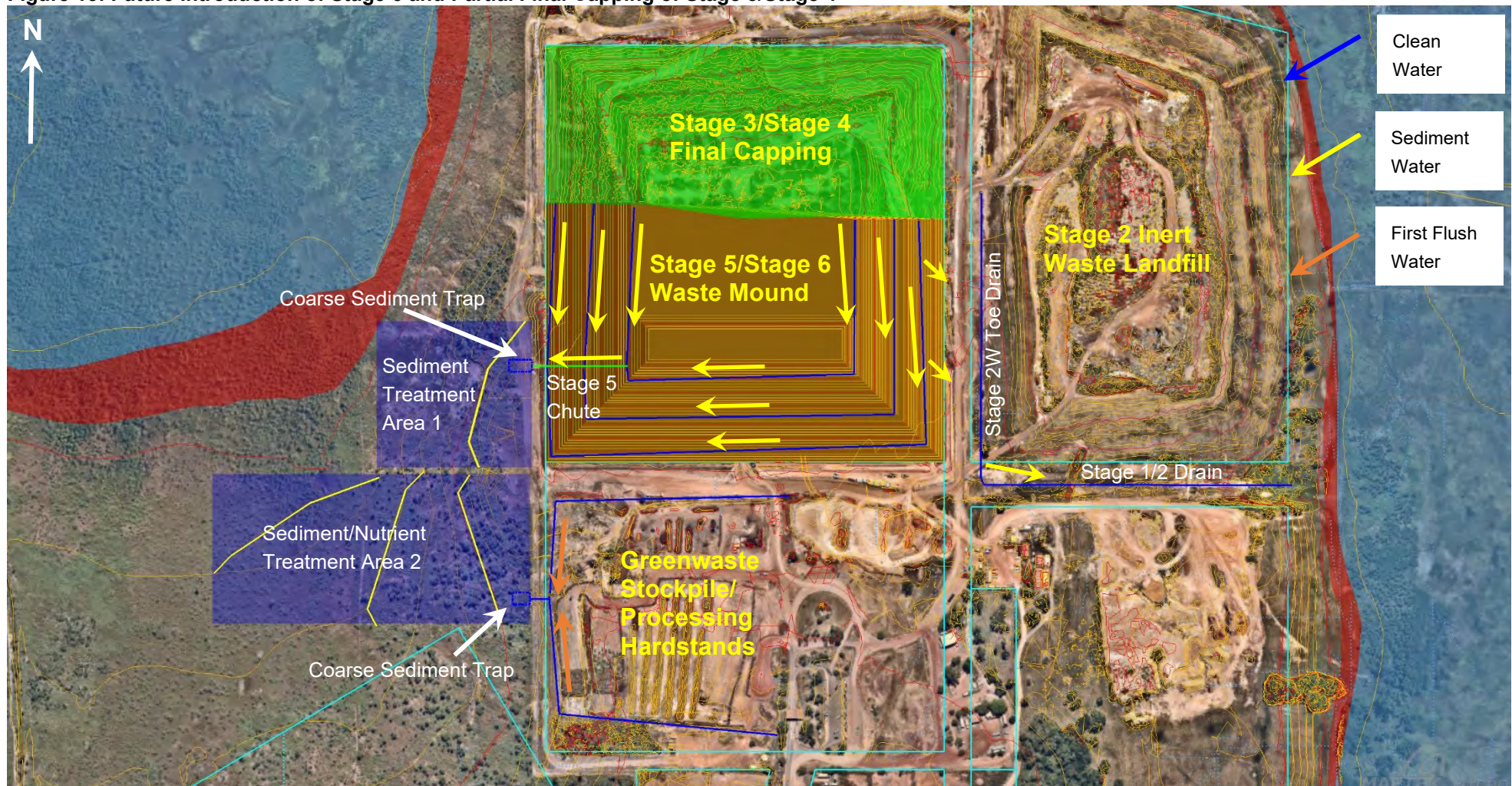
Figure 13: Future Introduction of Stage 6 and Partial Final Capping of Stage 3/Stage 4
