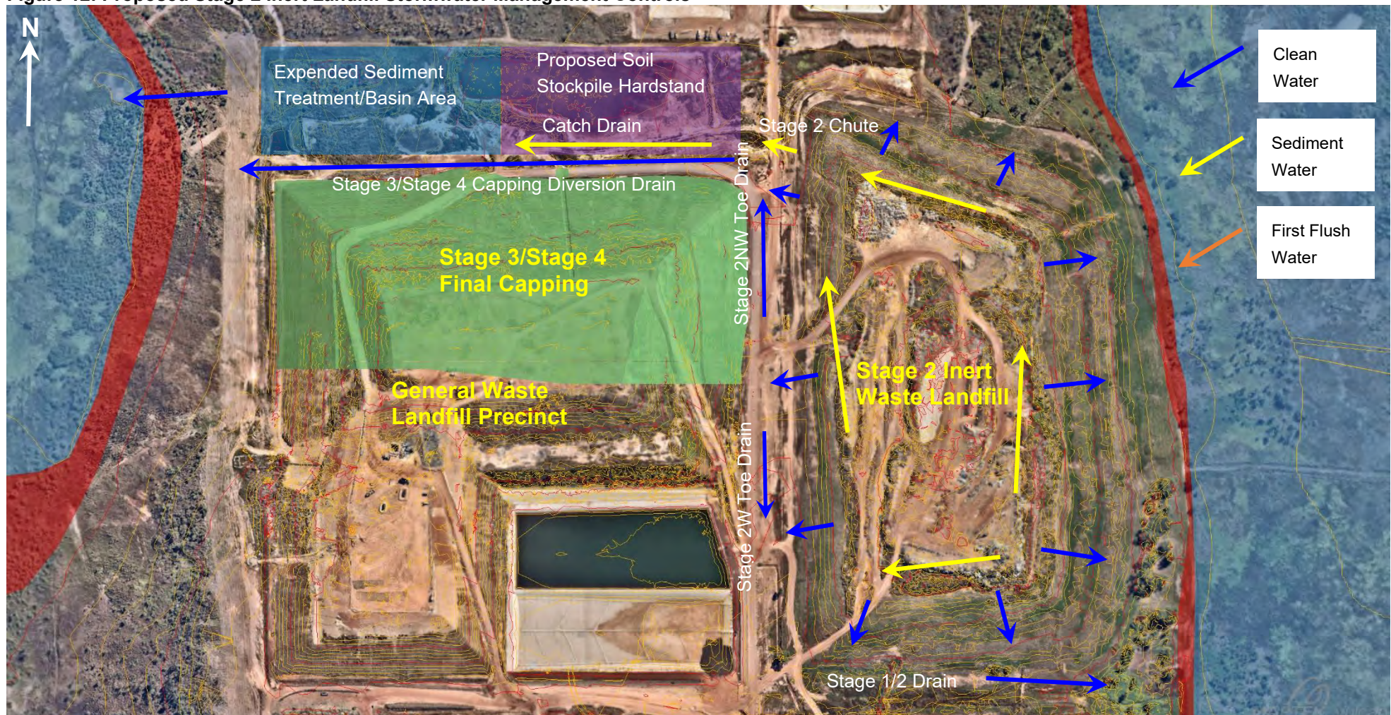
Figure 12: Proposed Stage 2 Inert Landfill Stormwater Management Controls
