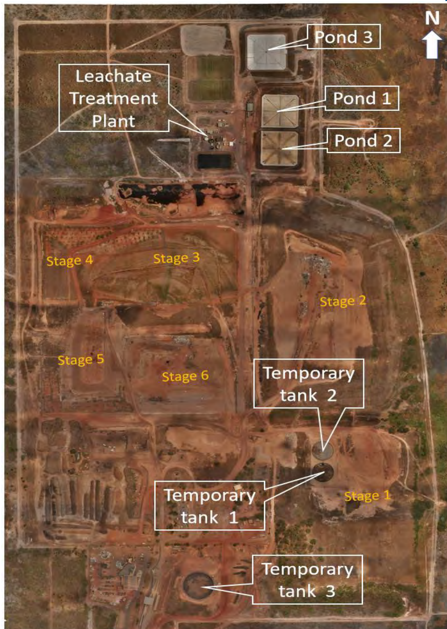
Figure 1: Leachate infrastructures at SBWMF.
