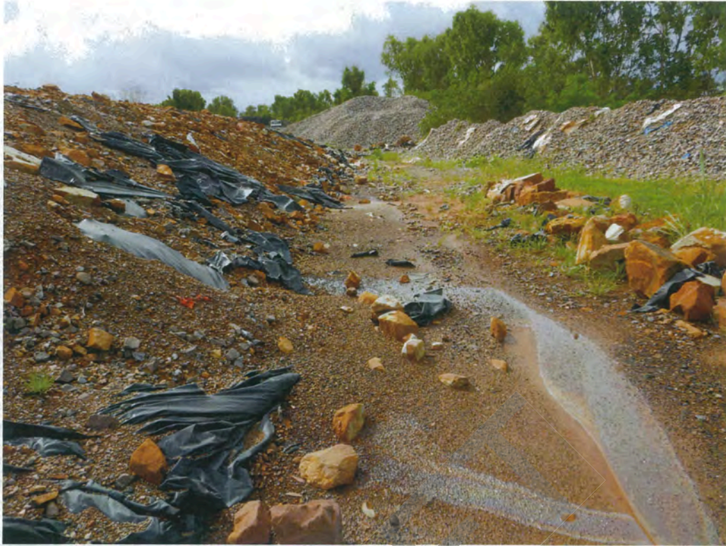
Photograph 3: Stockpiled material facing south. Visible hydrocarbon-like sheen leaching out of stockpile and pooling in surface water adjacent the stockpile.
