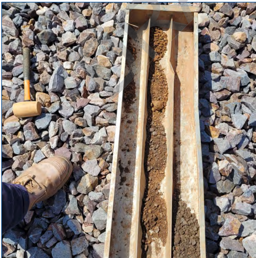
Photograph 2: View of silty clay sand material encountered in Area 1
