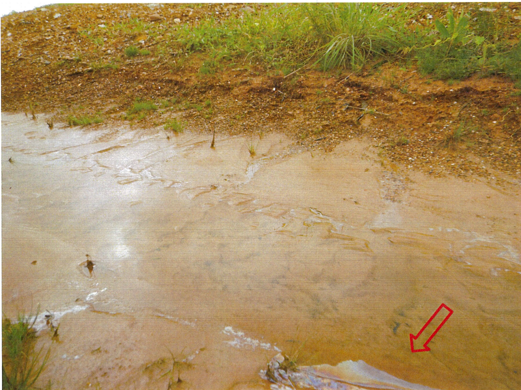
Photograph 6: Earthen stormwater drain located north of the stockpile. Visible hydrocarbon-like sheen visible in water and on surrounding ground surfaces.
