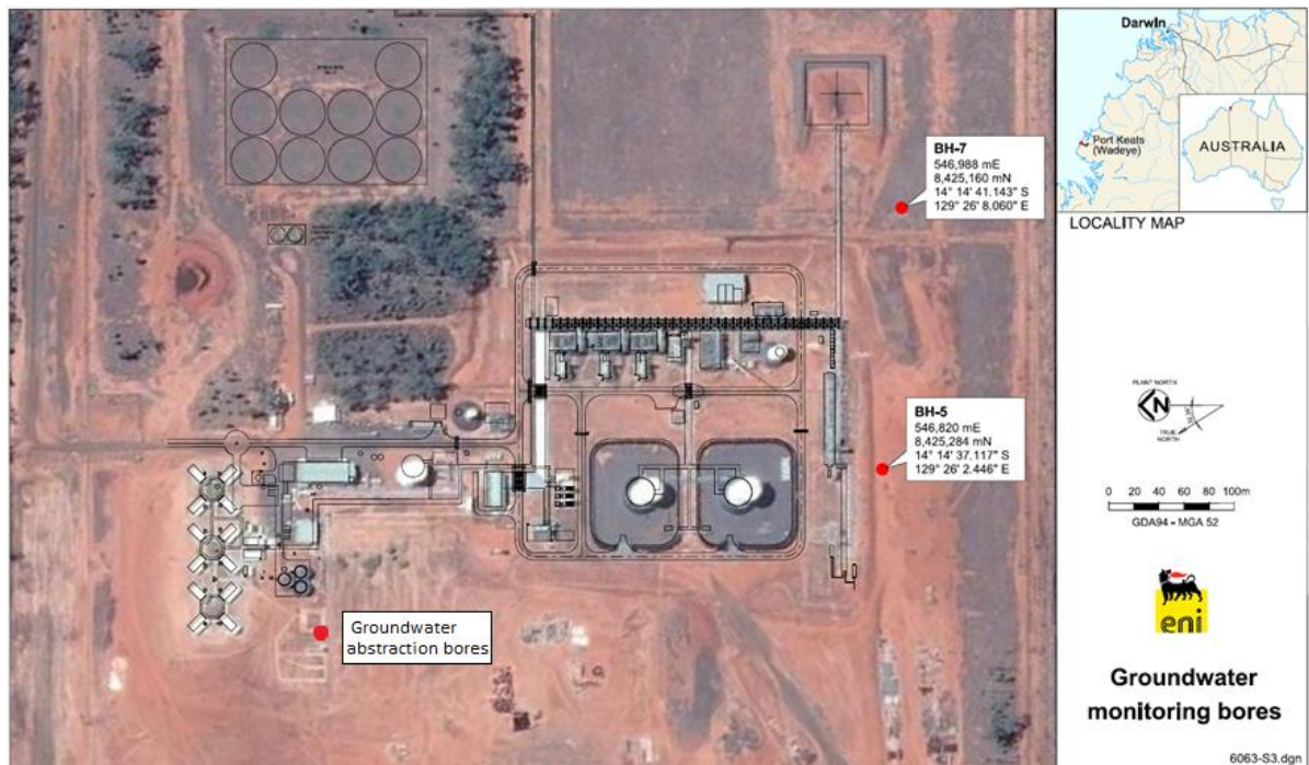
Figure 8.1: Groundwater abstraction and monitoring bores
