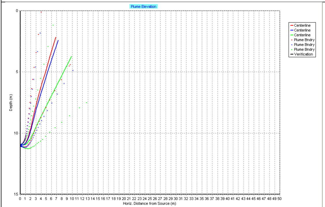
Figure 7.4: Case 1 (low 0.05 m/s currents under well mixed conditions) UM3 predictions where the red, green and blue line demarcate PFW salinities of 0.4, 5.0 and 20.0 psu
