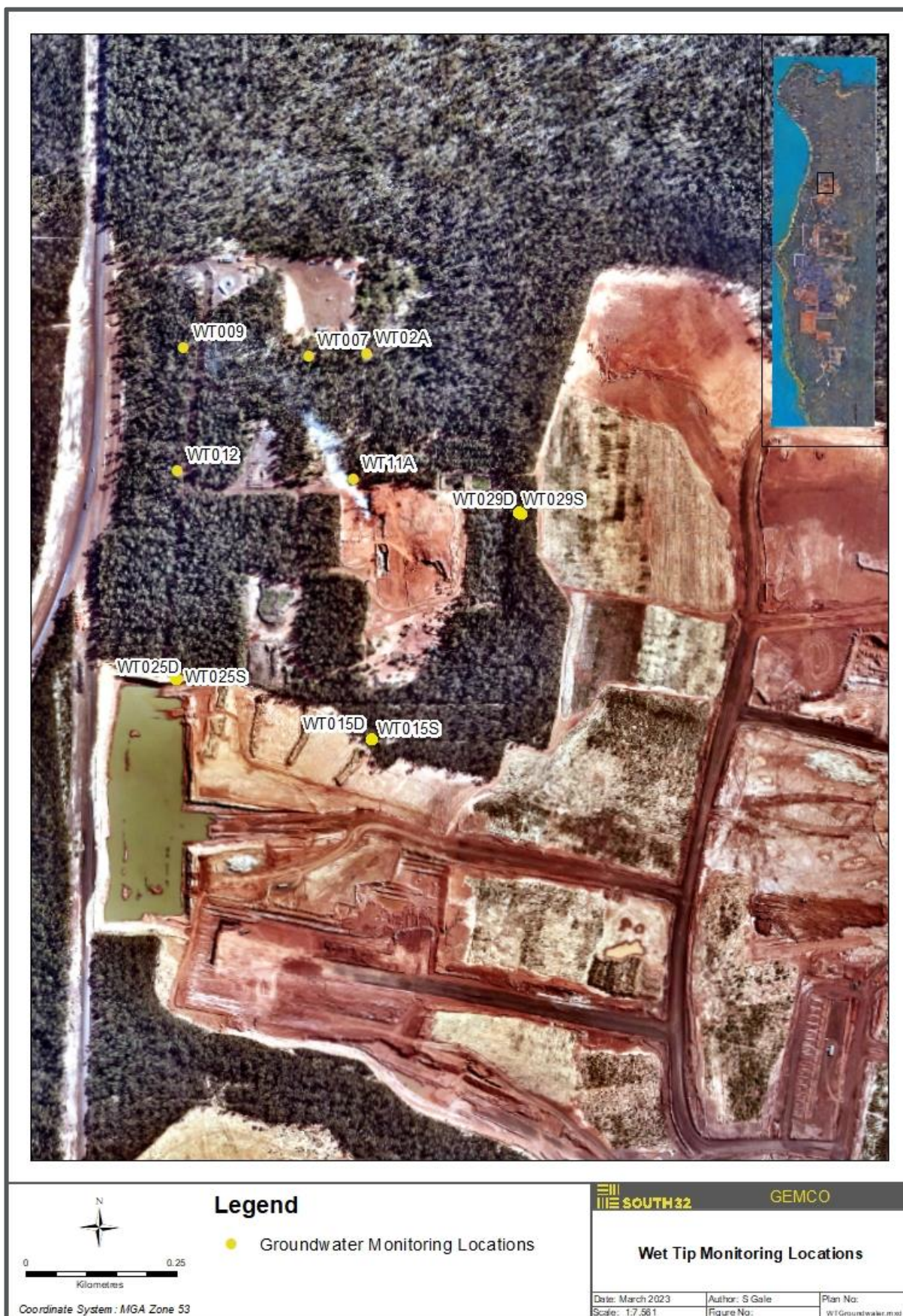
Figure 1: Groundwater monitoring network associated with Waste Management Facility
