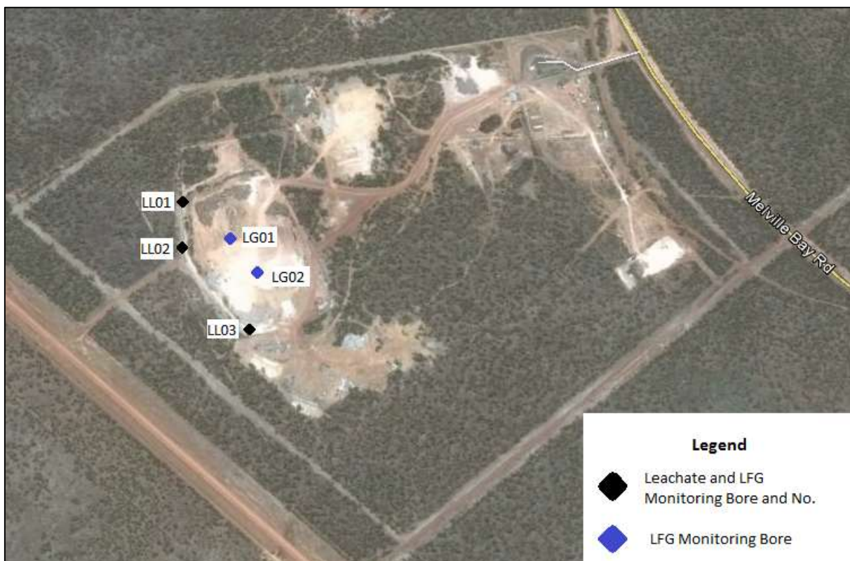
Figure 4: Landfill Gas Monitoring Bores installed at Gove Peninsula Waste Management Facility.
