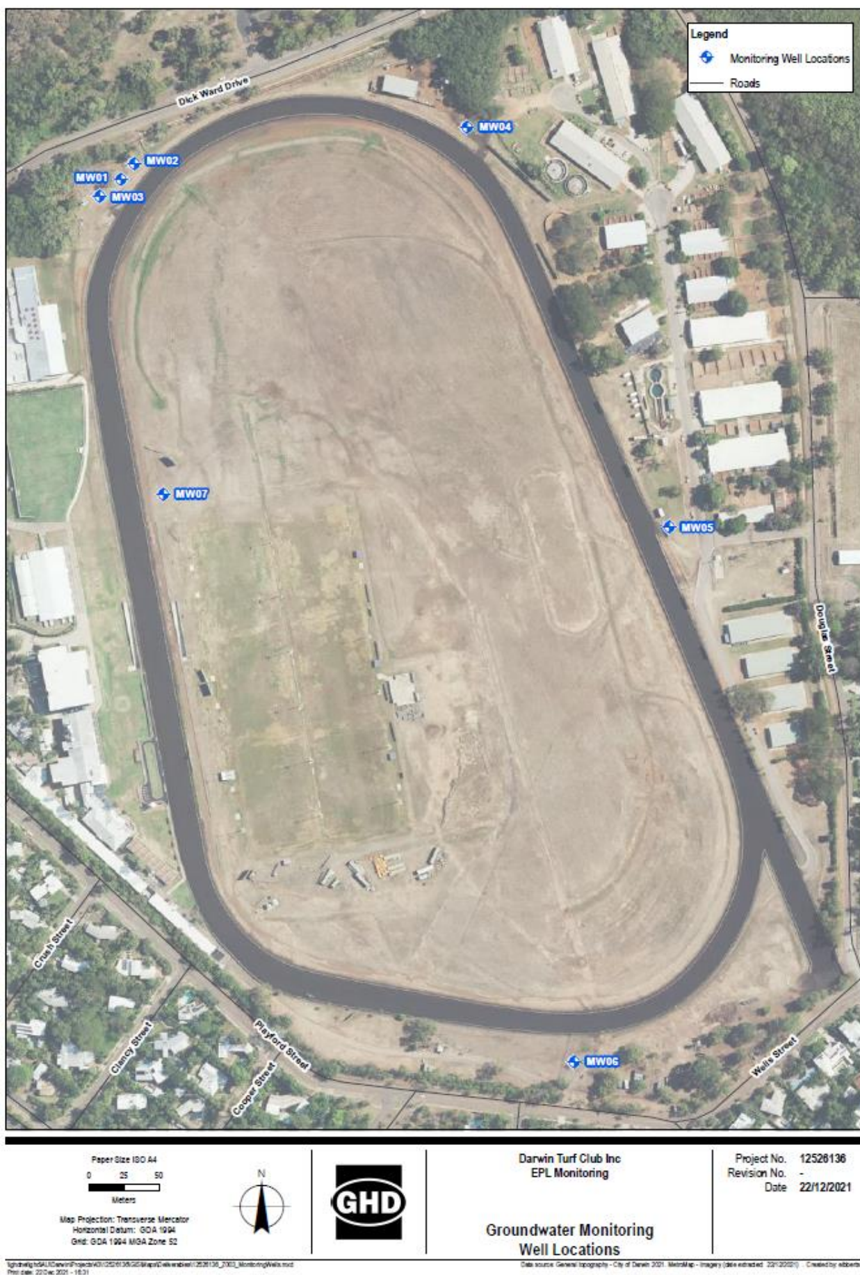
Figure 3 Groundwater monitoring well locations
