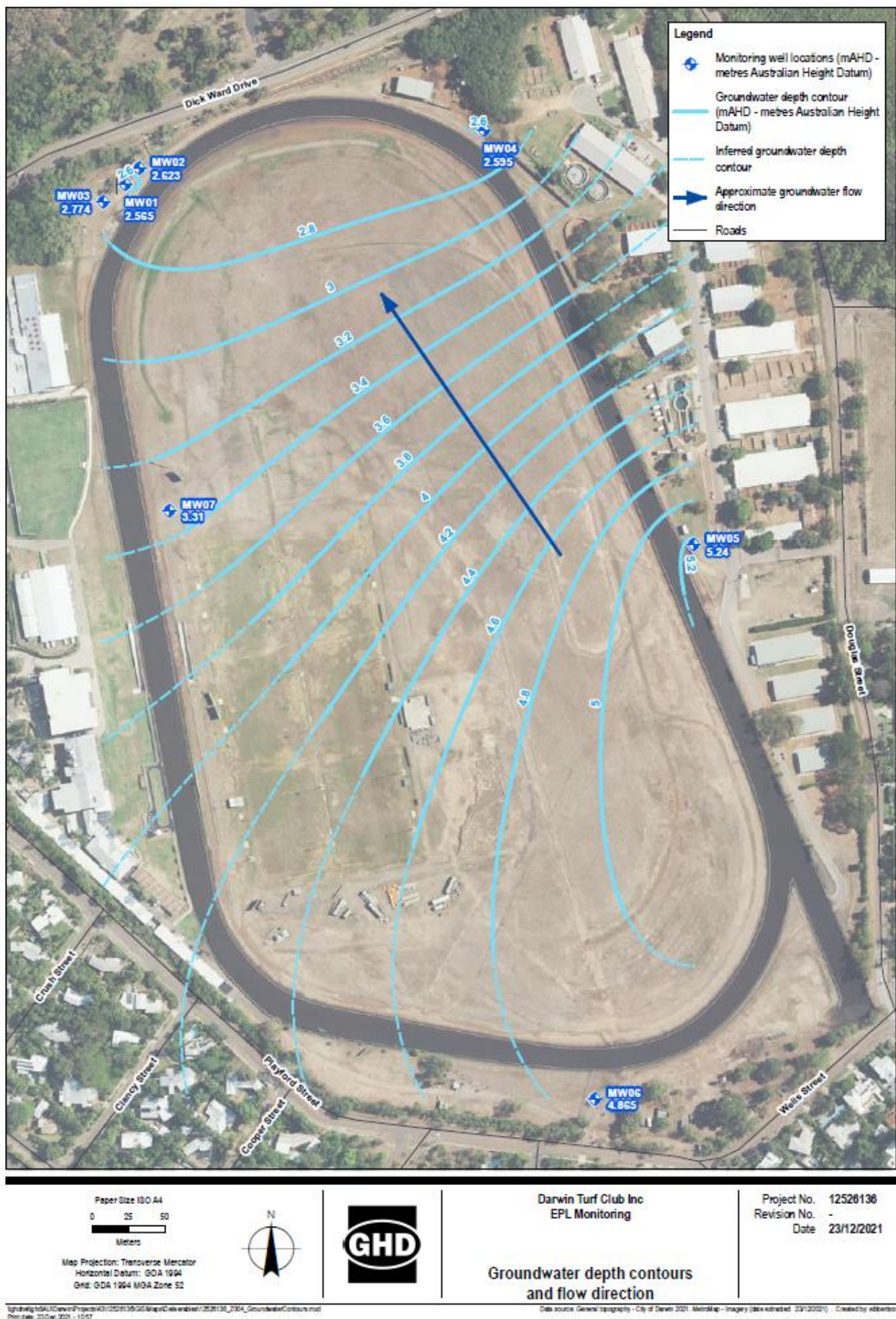
Figure 2 Groundwater depth contours and flow direction
