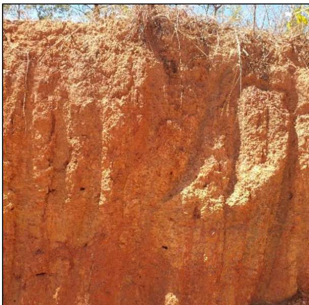
Figure 5.2 - Photo of lateritic soil profile typical at the site
