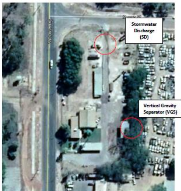
Figure 4-2 Location of Stormwater Sampling Locations – Katherine Facility
