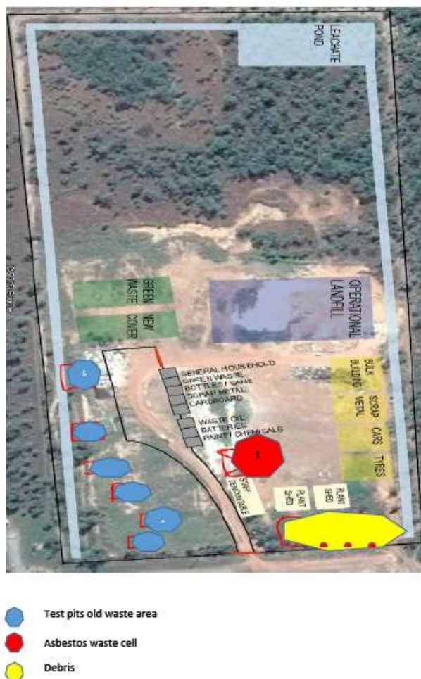
Figure 9: Location of test pits for old waste, asbestos waste and debris on the JWMF.
