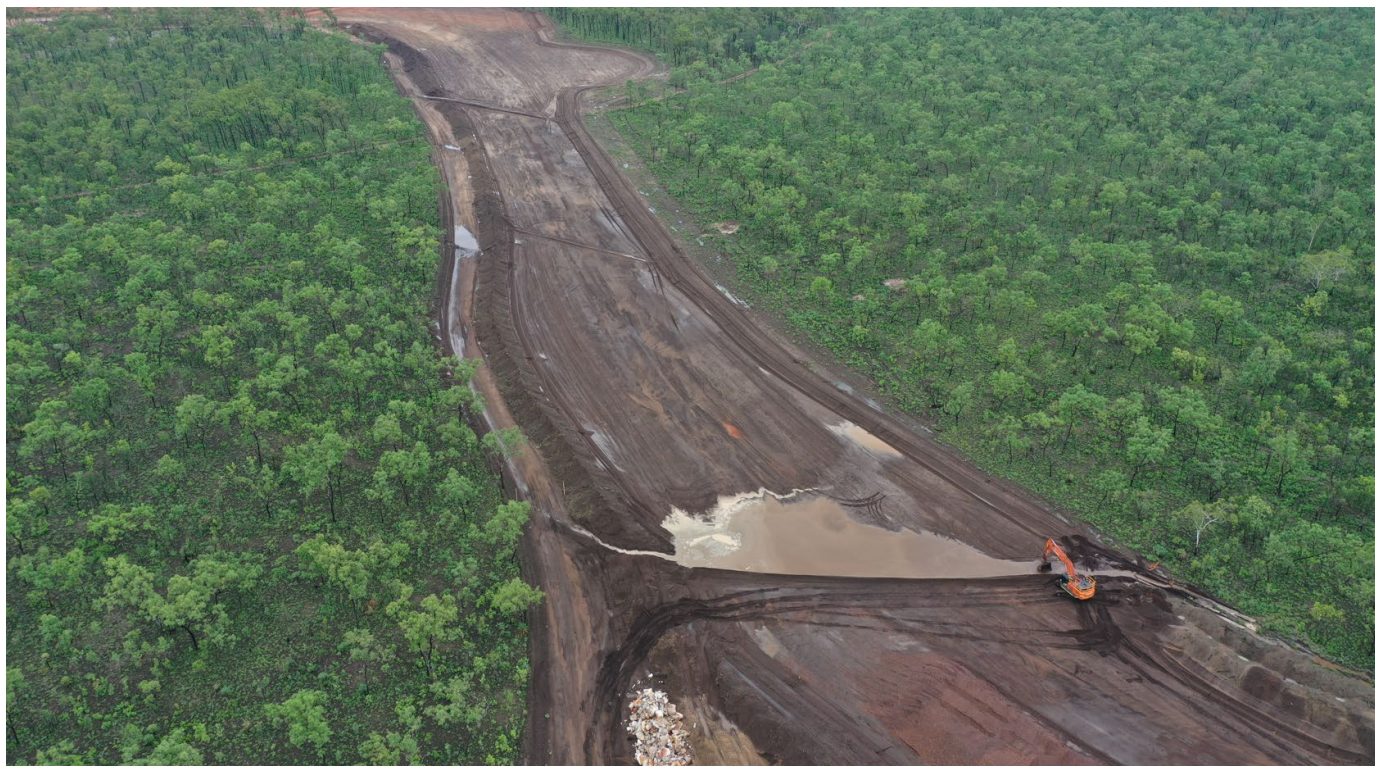
Figure 6: Improved frequency and size of diversion bunds in the catchment to the main Emerald River channel in response to the rainfall event on the 12/11/22.
