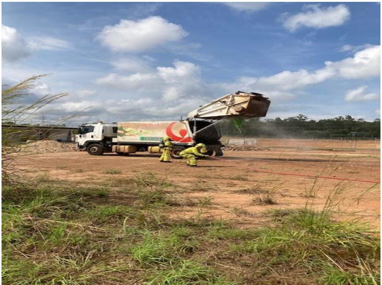
Figure 2: Truck was parked on the nearby vacant land where the waste was ejected and fire department personnel extinguished the flames.
