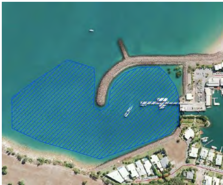
Figure 1- Overview of Dredge Footprint – Cullen Bay.
