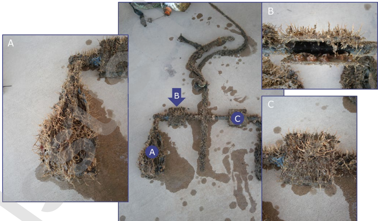
Figure 5-3: Example of monitoring photographs taken during monthly inspection a) rope mop, b) inside the plates and c) plates surface biofouling conditions
