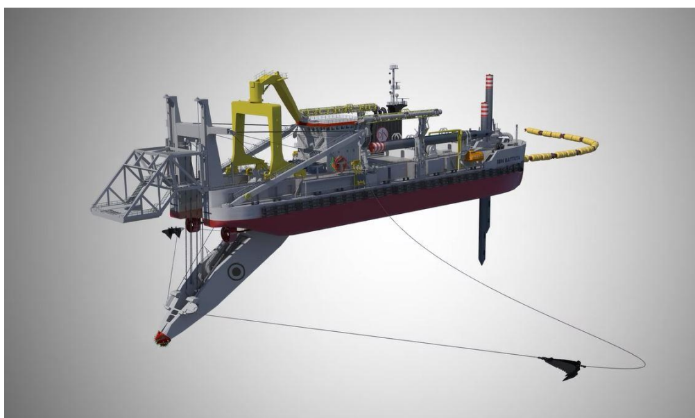
Figure 3-2 Example of a Cutter Suction Dredger (CSD)
